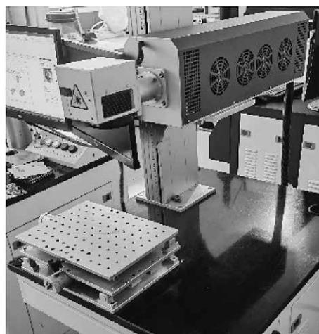
Figure 1 Laser marking machine
