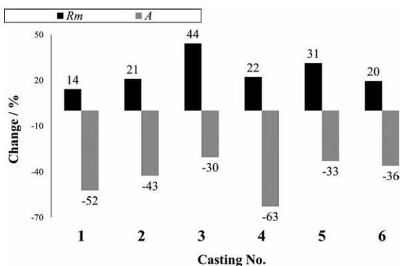
Figure 1 Change in mechanical properties calculated according to formula 1 for wire rod number from 1 to 6
