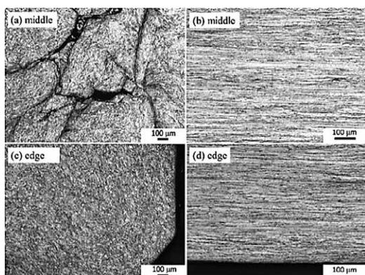
**Figure 6** Microstructure of wire rod number 7 total draft 91,3 %, a, c - cross section, b, d - longitudinal section
