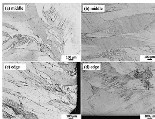
Figure 3 Microstructure of wire rod number 4, total draft 57,2 %, a, c - cross section, b, d - longitudinal section
