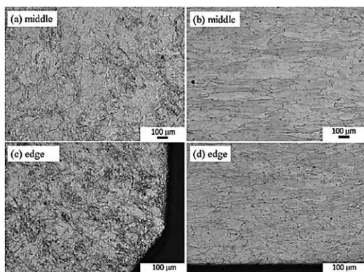
**Figure 5** Microstructure of wire rod number 7 total draft 57,2 %, a, c - cross section, b, d - longitudinal section
