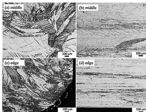
Figure 4 Microstructure of wire rod number 4, total draft 91,3 %, a, c - cross section, b, d - longitudinal section
