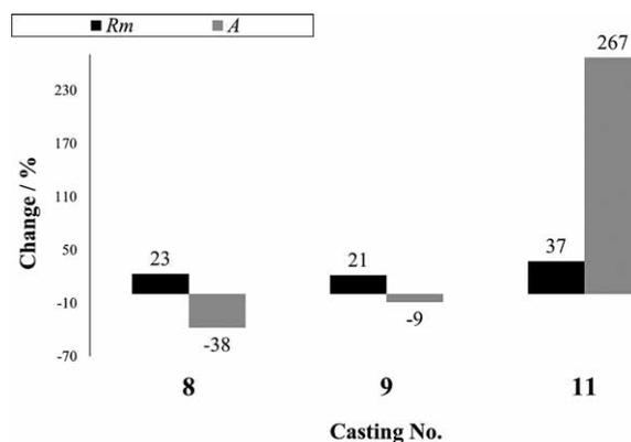
Figure 2 Change in mechanical properties calculated according to formula 1 for wire rod number 8, 9 and 11
