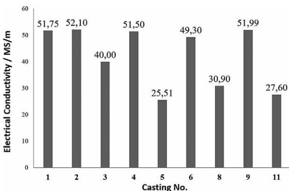
**Figure 7** Electrical conductivity depending on chemical composition, total draft 91,3 %
