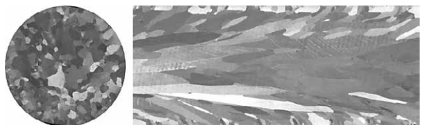
Figure 6 CuMg0.05 alloy macro-structure
