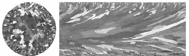
Figure 7 CuMg0.2 alloy macro-structure
