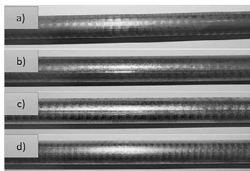
Figure 2 Exemplary pictures of the obtained rods: a) CuMg0.02, b) CuMg0.05, c) CuMg0.2, d) CuMg0.5
