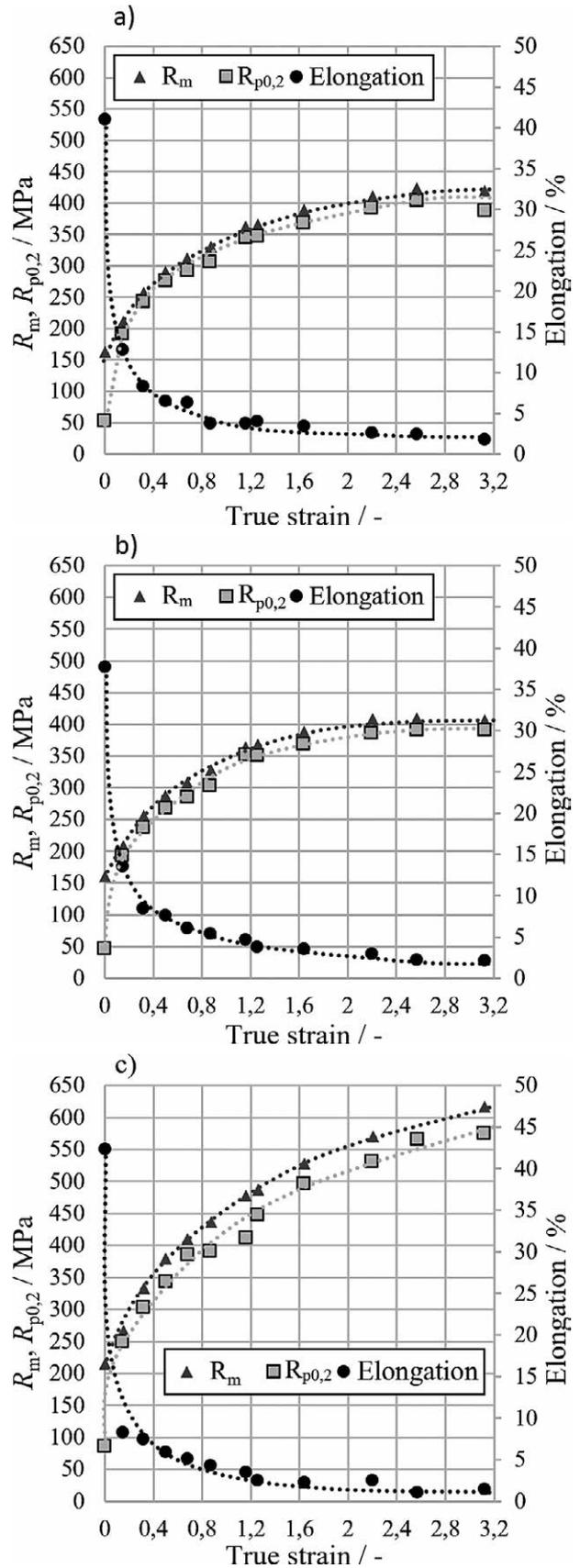
Figure 2 Work-hardening curves obtained in cold drawing process of previously casted rods: a) CuMg0.02, b) CuMg0.05 and c) CuMg0.5 alloys
