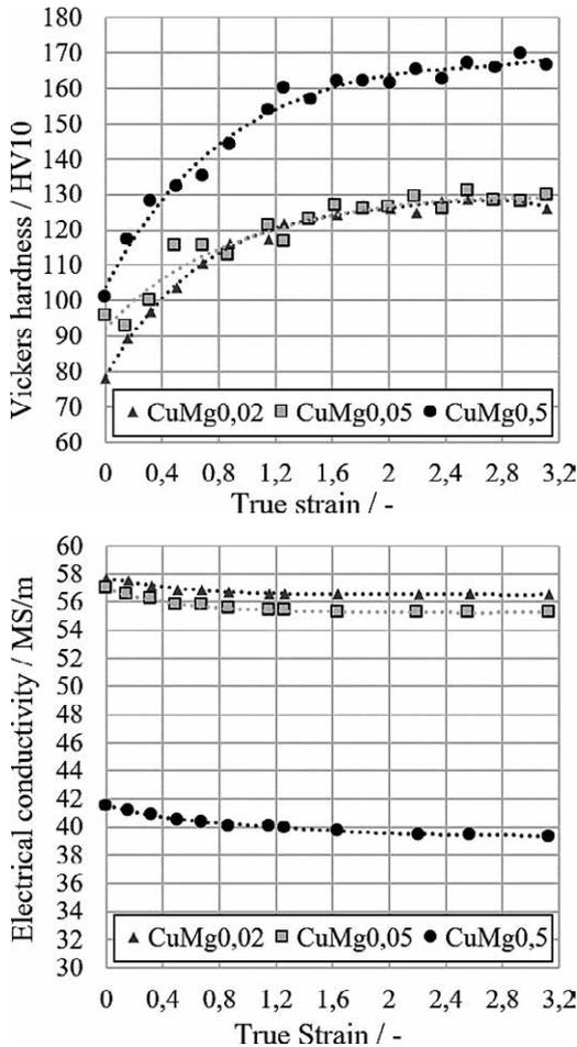
Figure 1 Vickers hardness and electrical conductivity research results for all Cu-Mg materials at all staged of cold drawing process from 9,38 mm to 1,97 mm diameter.
