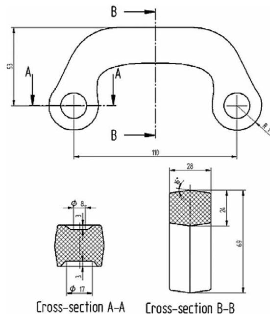
**Figure 6** Characteristic dimensions of the preform by variant no. 3
