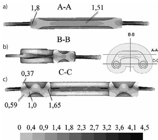
**Figure 12** Distribution of strain in the cross sections of the connector forged using preform no. 3: a) along the shaft groove, b) perpendicular to the shaft groove, c) through the middle of the heads
