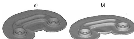
Figure 10 The shape of the connector forged using the preform by variant: a) no. 2, b) no. 3
