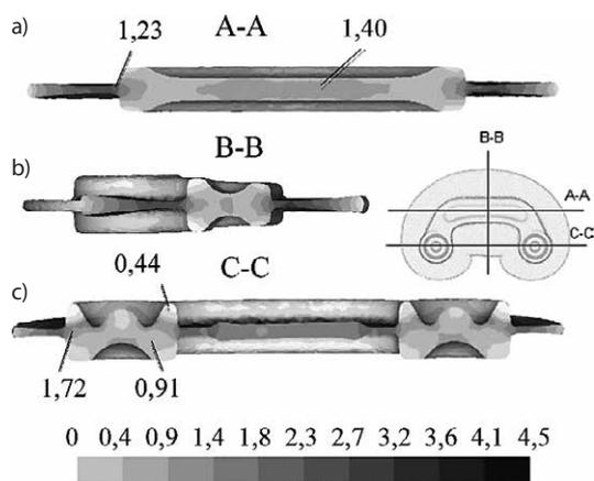
Figure 8 Distribution of strain in the cross section: a) along the shaft groove, perpendicular to the shaft groove, c) through the middle of the heads
