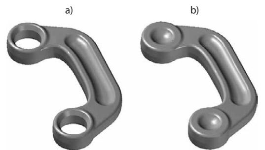
**Figure 1** Models 3D of the analyzed connector: a) finished part, b) forging
