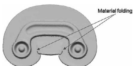
Figure 7 The shape of the connector forged using the preform by variant 1 and folds detected
