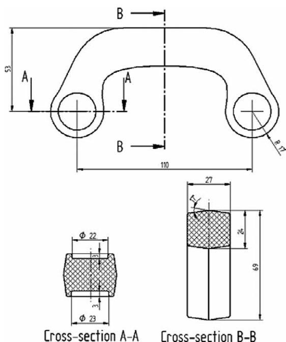
**Figure 4** Characteristic dimensions of the preform by variant no. 1
