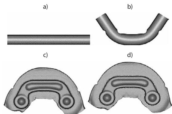
**Figure 2** Current forging technology for connector: a) cylindrical billet; b) shape obtained in the bending operation; c) shape obtained in the preliminary die forging; d) shape obtained in finishing die forging
