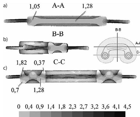
Figure 11 Distribution of strain in the cross sections of the connector forged using preform no. 2: a) along the shaft groove, b) perpendicular to the shaft groove, c) through the middle of the heads
