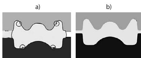
Figure 9 Cross section of the connector head showing a) folds created in the earlier deformation stage, and b) their disappearance due to remeshing later
