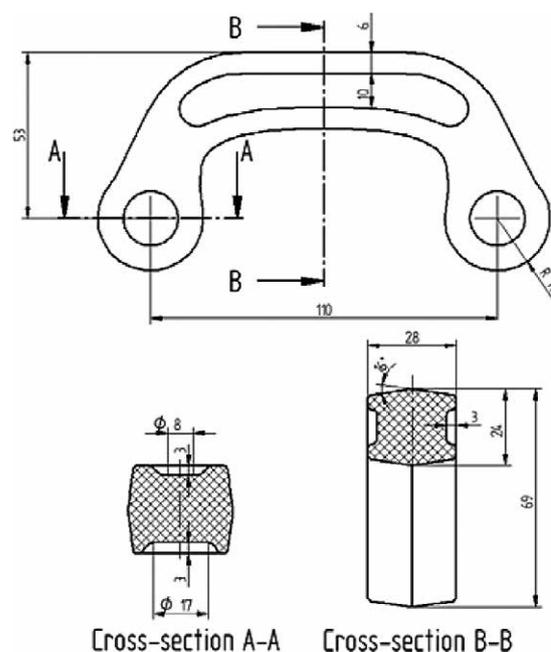
**Figure 5** Characteristic dimensions of the preform by variant no. 2
