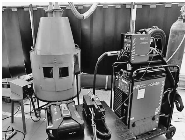
Figure 1 Testing station for fume emission measurements during arc welding [10]
