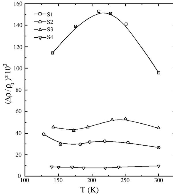
Fig. 1. Temperature variation of magnetoresistance of samples S<sub>1</sub>, S<sub>2</sub>, S<sub>3</sub> and S<sub>4</sub>, of bismuth.
