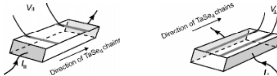
Fig.1. Sketch of the sample geometry and the contact configurations for the electrical conductivity measurements.
