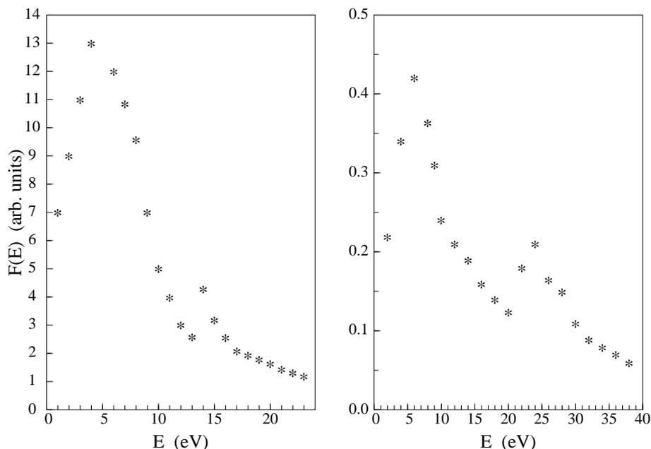
Fig. 4. Electron energy distribution function in the cathode fall region, discharge in Ar,  $P = 130$  Pa (1.0 torr) and  $I_A = 10$  mA.
