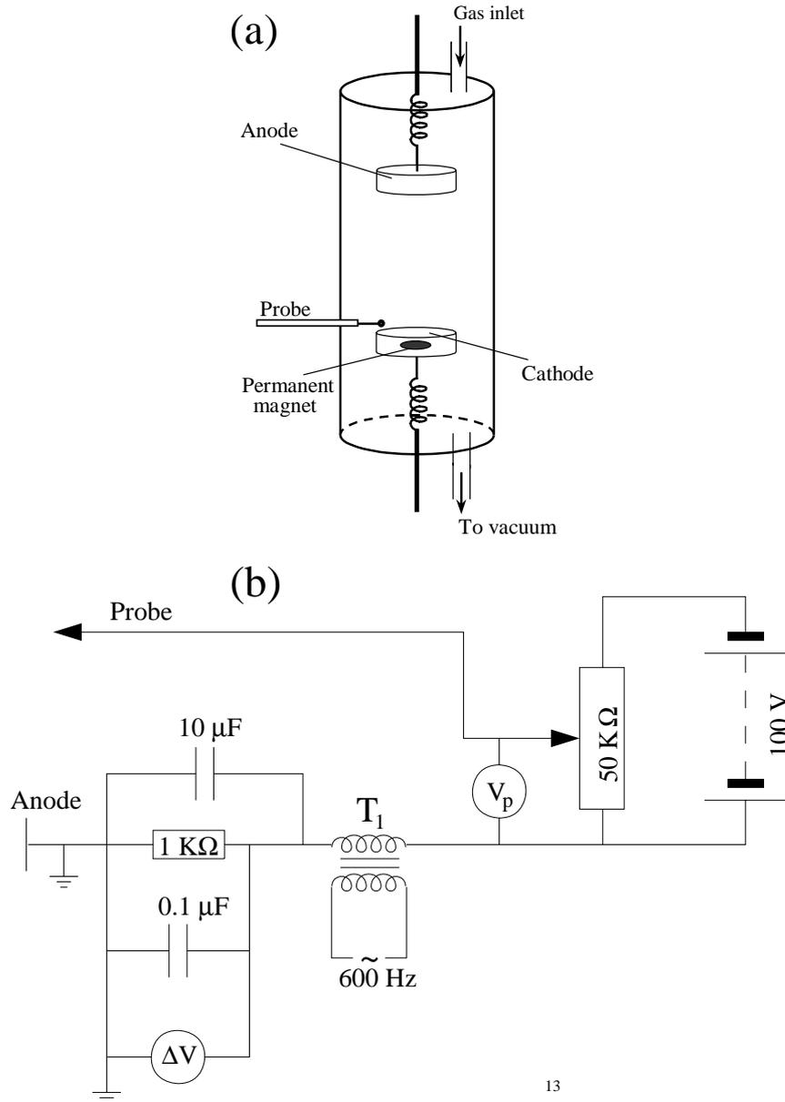
Fig. 1. a) Schematic drawing of the DC magnetron used in the measurements. b) Block diagram of the electronic circuit.
