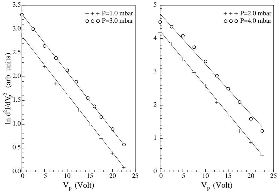
Fig. 6. Dependence of the second derivative of the electron current on the probe voltage, discharge in the positive column region in Ar, anode current 10 mA.
