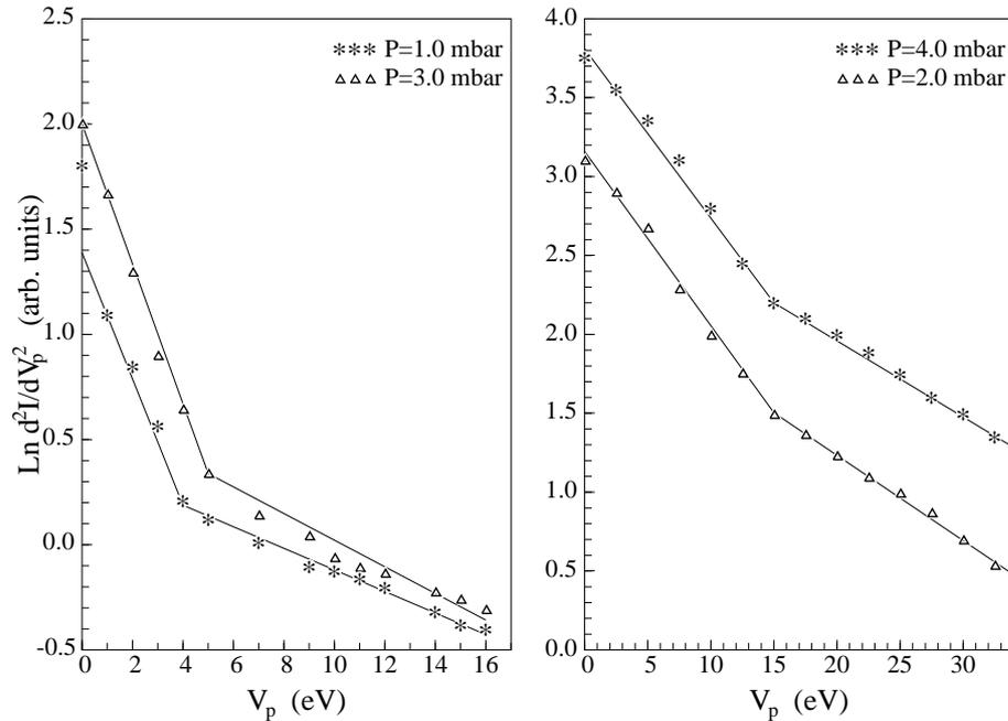
Fig. 2. Dependence of the second derivative of the electron current on the probe voltage, discharge in the cathode fall region in Ar, anode current 10 mA.
