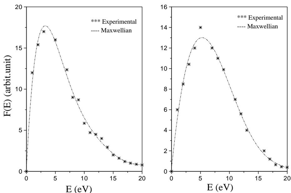
Fig. 8. Electron energy distribution function in the positive column region, discharge in Ar,  $P = 130$  Pa (1.0 torr) and  $I_A = 10$  mA.
