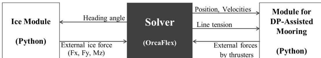
**Fig. 1** Example of dynamic motion analysis with ice and DP modules in the time domain with a motion solver [10]
