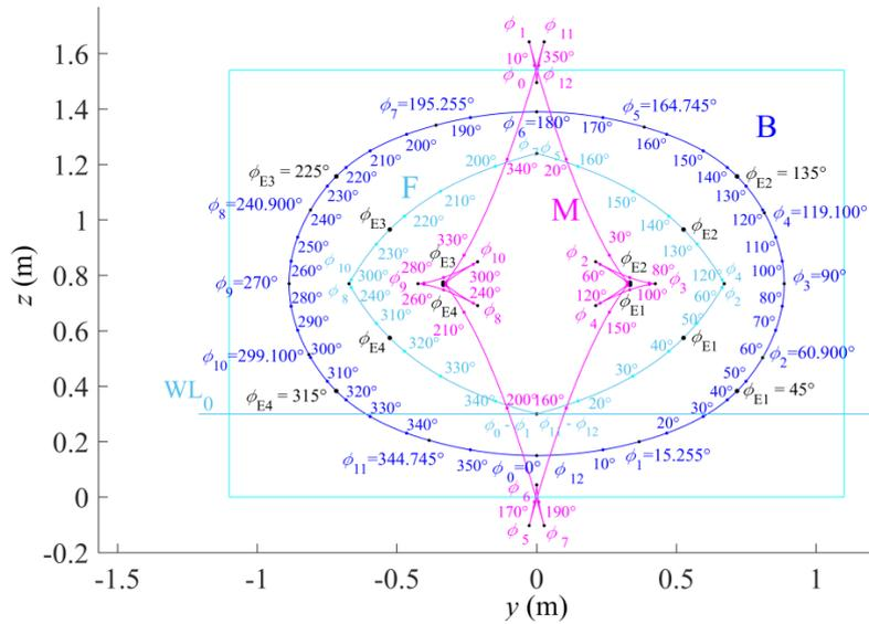
**Fig. 9** Hydrostatic properties for rectangular cross section pontoon, for  $d = 0.3$  (m)
