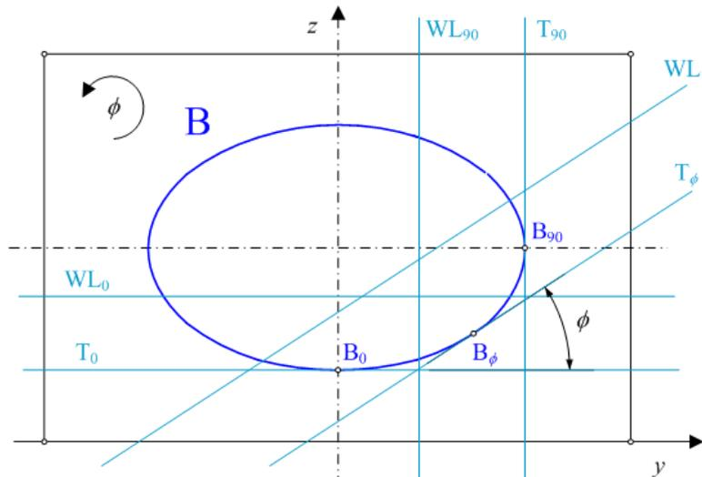
**Fig. 6** Centre of buoyancy B-curve tangents parallel to inclined waterline
