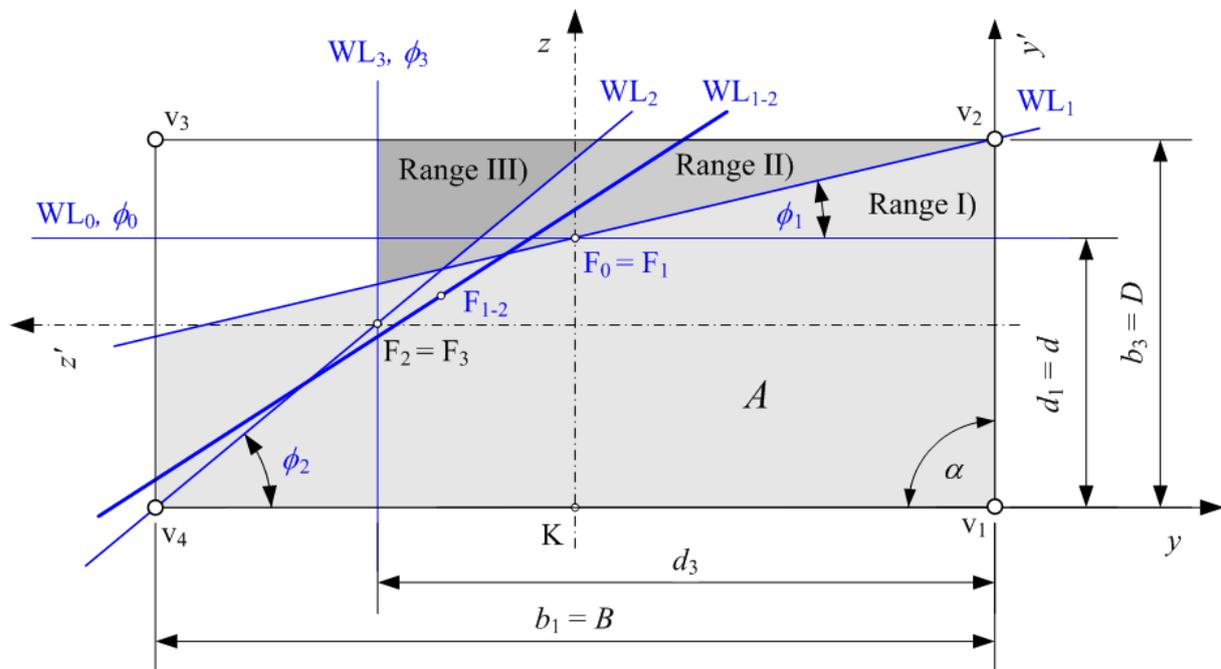
**Fig. 1** Rectangle calculation regions defined by deck immersion/bottom emersion heel angle ranges
