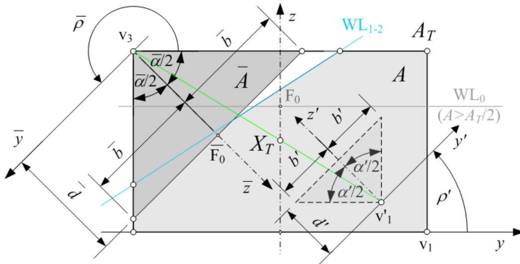
**Fig. 5** Isosceles triangle as hydrostatic cross section area complement of rectangular pentagon, with its scaling
