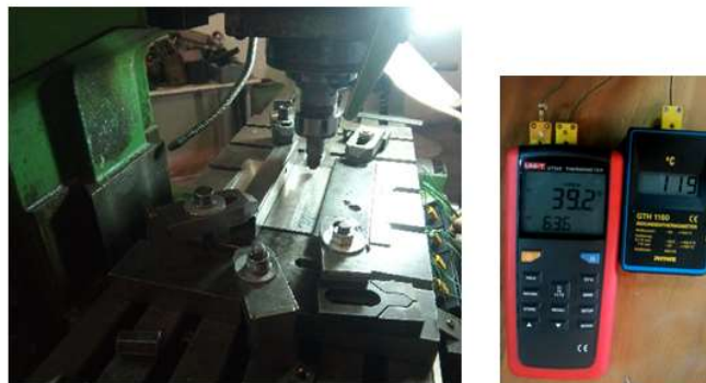
Figure 4. Position of thermocouples used in this investigation.
