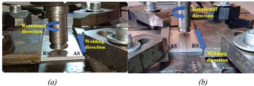
Figure 3. Stir welded Lap joint, (a) Configuration (A), (b) Configuration (B).
