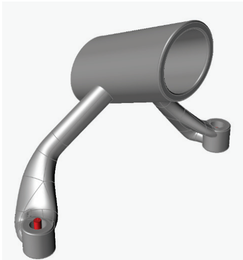
Figure 15 Post-processed topology optimized design (minimized mass) [11]
