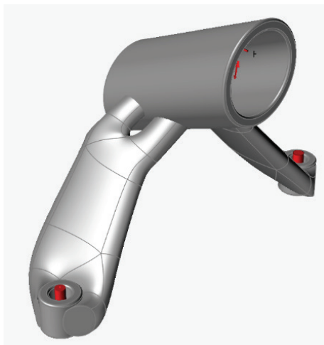
Figure 20 Post-processed topology optimized design (max. stiffness) [11]
