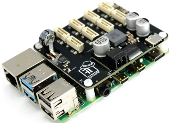
Figure 2 HAT module installed on the top of the Raspberry Pi board
