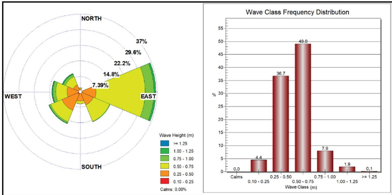
Fig 6. The wave characteristics were significant during 2006-2019; Waverose (left); Distribution of high-frequency waves (right)
