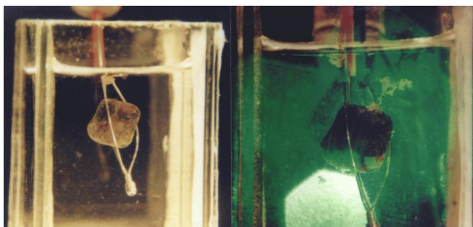
Fig. 1. (top) The experimental setup for shadowgraphy. (bottom left) Photograph of the stone. (bottom right) The shadowgraph of the stone made with a 7 ns N-Dye laser pulse.
