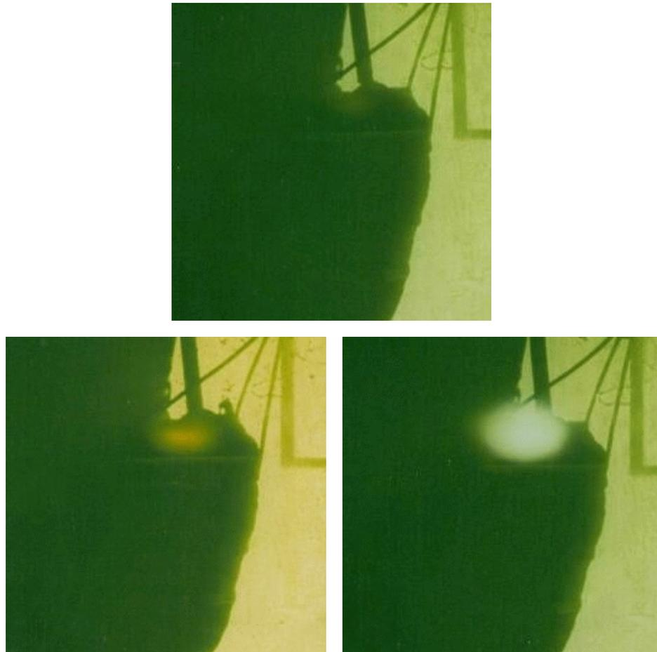
*Fig. 2. Time-resolved shadowgraphy when the tip of the fiber was touching the surface of the stone.*
