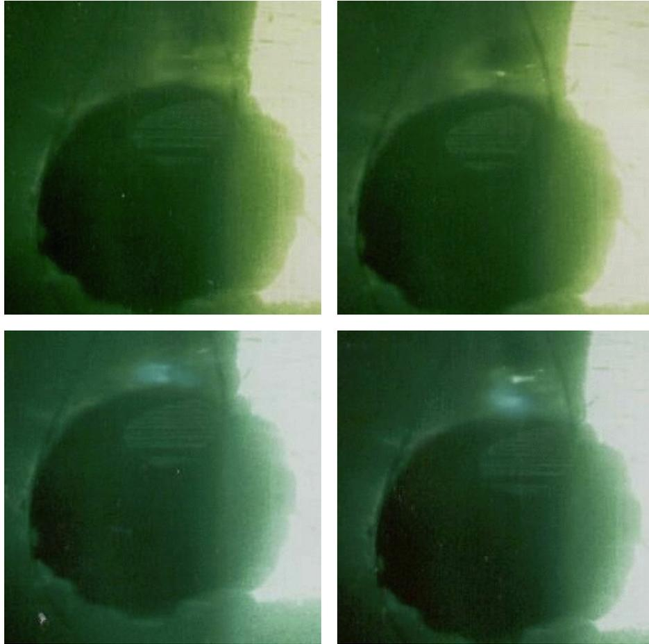
*Fig. 3. Time-resolved shadowgraphy when the tip of the fiber was at the distance of 7 mm from the stone.*
