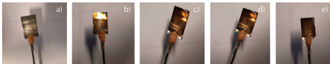
Fig. 4 – Pt electrode with deposited Cu layer from \text{CuSO}_4 \cdot 5\text{H}_2\text{O} solutions of different concentrations: a) 1.0, b) 2.5, c) 5.0, d) 7.5, and e) 10.0 mM
