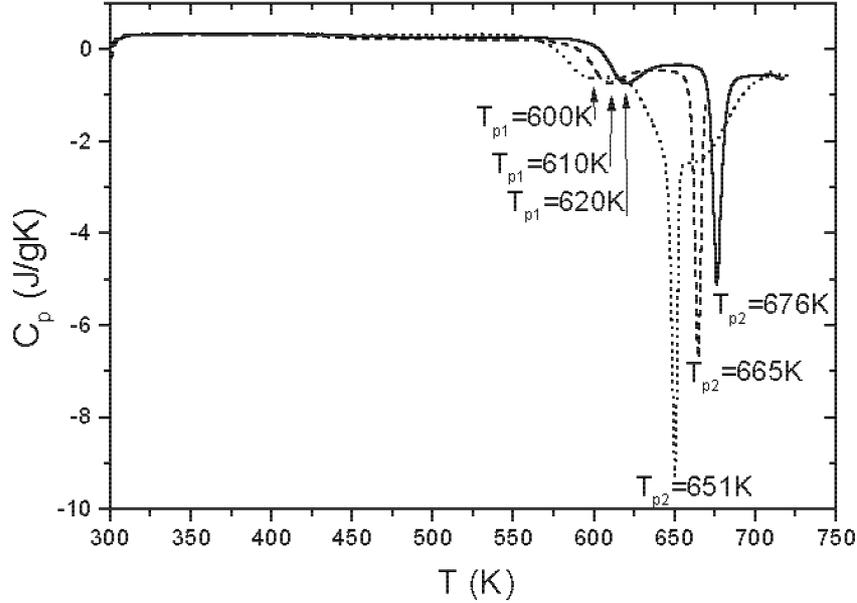
Fig. 1. The temperature dependence of  $C_p$  of the  $Zr_{80}Co_{20}$  metallic glass in the temperature range of 298 – 723 K at the heating rates,  $s$ :  $s = 60$  K/min (full line),  $s = 30$  K/min (dashed line),  $s = 10$  K/min (dotted line).
