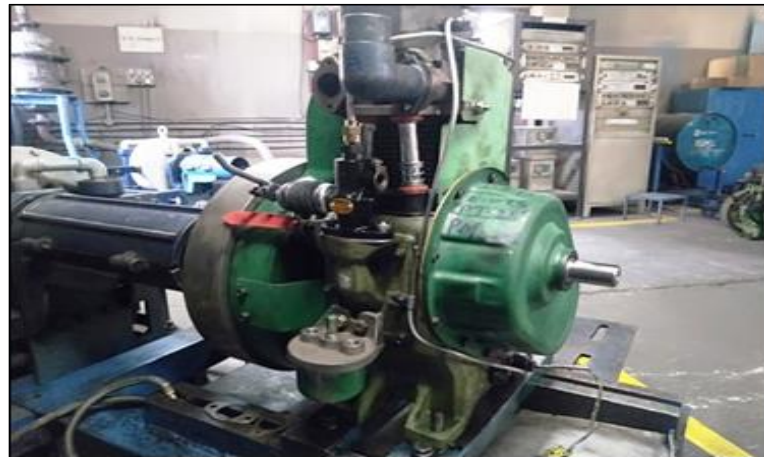
Figure 9. Testing of the developed fuel filter cap on engine testing set up.
