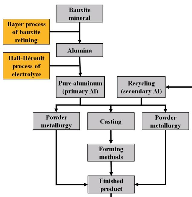
Fig.12. Flow chart of Al production process [57]
