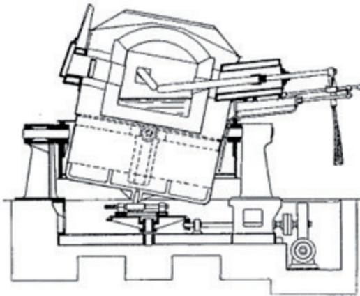
Fig. 4. Stassano furnace [48]
