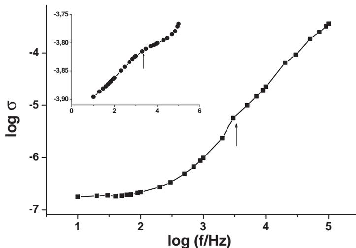
Fig. 5. Conductivity plot of pure mangosteen (■), inset curve for orthophosphoric acid complex of mangosteen (●). Calculated values are at RT.
