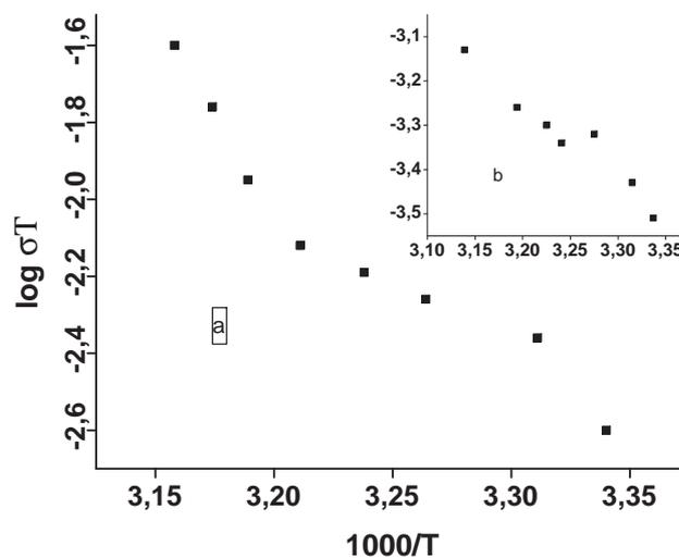
Fig. 6. Arrhenius plot for the pure mangosteen (■), inset curve for orthophosphoric acid complex of mangosteen (◆). Applied voltage of 1 V AC at frequency 5 kHz.
