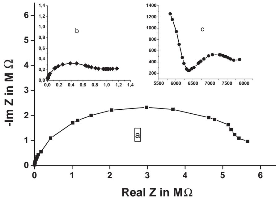
Fig. 4. Impedance plot of (a) pure gum mangosteen, (b) mangosteen gum-acetic acid complex (sample thickness 0.1535 cm, area 1.66 cm<sup>2</sup>) and (c) mangosteen-orthophosphoric acid complex (sample thickness 0.125 cm, area 2.54 cm<sup>2</sup>) at RT, applied p.d 1V (sample thickness 0.1525 cm, area 1.76 cm<sup>2</sup>), Z in Ω.
