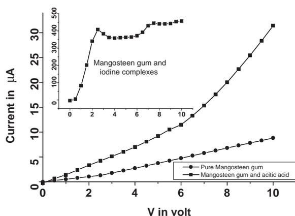
Fig. 3. DC  $V-I$  characteristics of pure mangosteen (■) (sample thickness 0.1525 cm, area 1.76 cm<sup>2</sup>), acetic acid complex of mangosteen (●) (sample thickness 0.1535 cm, area 1.66 cm<sup>2</sup>). Inset graph: iodine complex of mangosteen (■) (sample thickness 0.15 cm, area 1.72 cm<sup>2</sup>).
