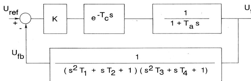
Fig. 3. Block diagram of the control loop.
