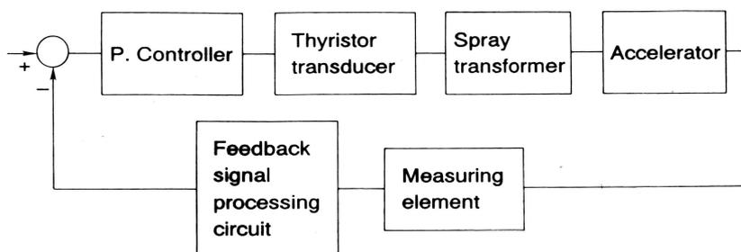
Fig. 2. Schematic diagram of the stabilization system.
