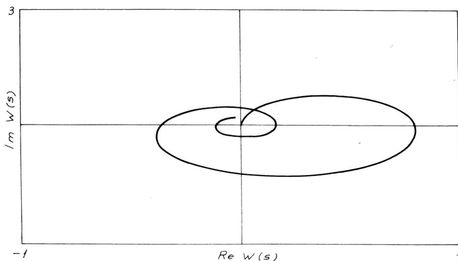
Fig. 4. Nyquist diagram of the stabilization system.
