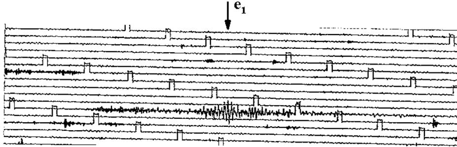
Fig. 3. The seismogram of the earthquake recorded at 25<sup>th</sup> June 1998, at 10 h 52 min, at the Medvednica Seismological Station of the Geophysics Department, University of Zagreb; horizontal distance between two neighbouring rectangular pulses denotes a time interval of 1 min.
