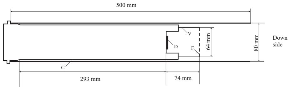
Fig. 1. Radon-emanation detector; C - cylinder, D - detector film, V - cup and F - filter.
