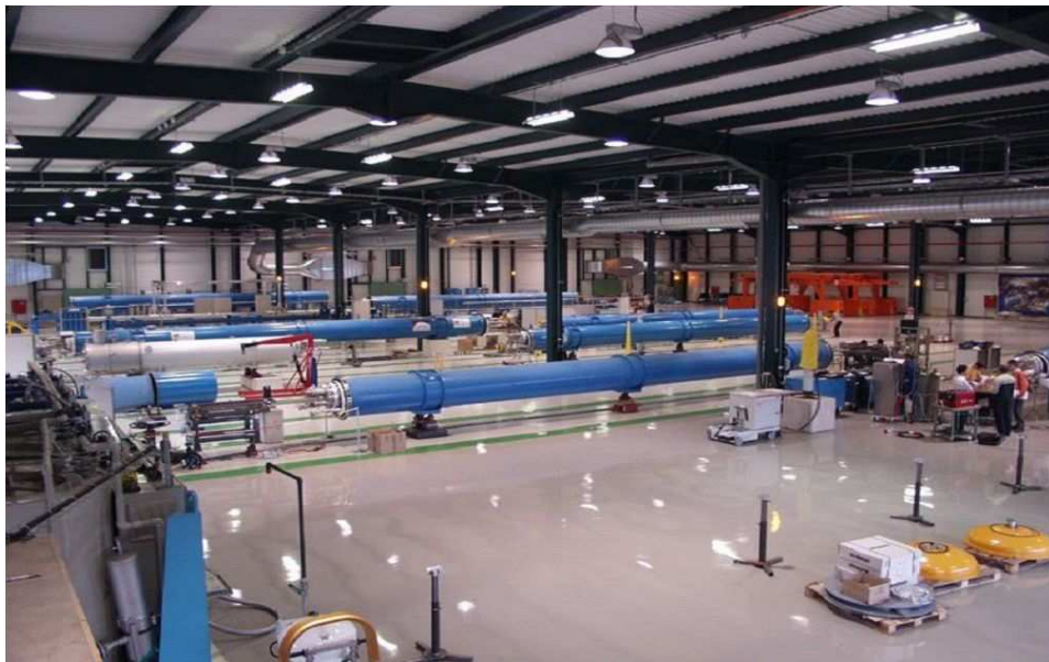
Fig. 5. Cryostating main dipoles at CERN.
