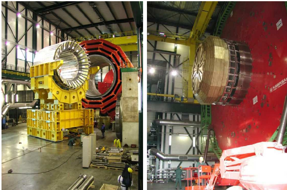
Fig. 20 (left). Half of the barrel hadron calorimeter in its cradle, prepared for test installation.
