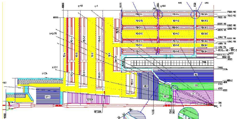
Fig. 8. Longitudinal cut through one quadrant of CMS; the barrel and endcap muon stations are denoted by MB and ME, the tower structure of the hadron calorimeter (HB, HE) and the arrangement of the electromagnetic calorimeter crystals (EB, EE) is indicated.
