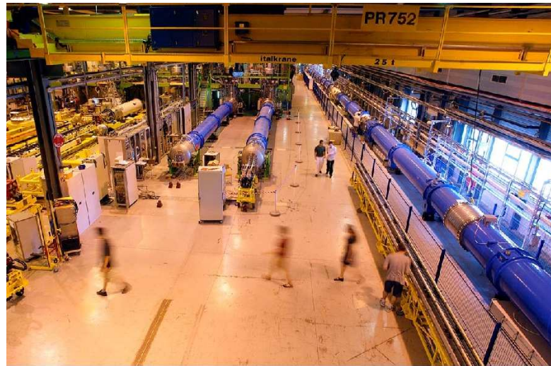
Fig. 7. LHC dipoles on test benches (center/left) and the LHC string test (right).
