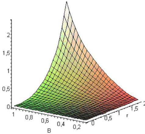
*Fig. 1. Dependence of the energy (ordinate, according to Eq. (14)) and strength of magnetic field ( $B$ ) on distance.*
