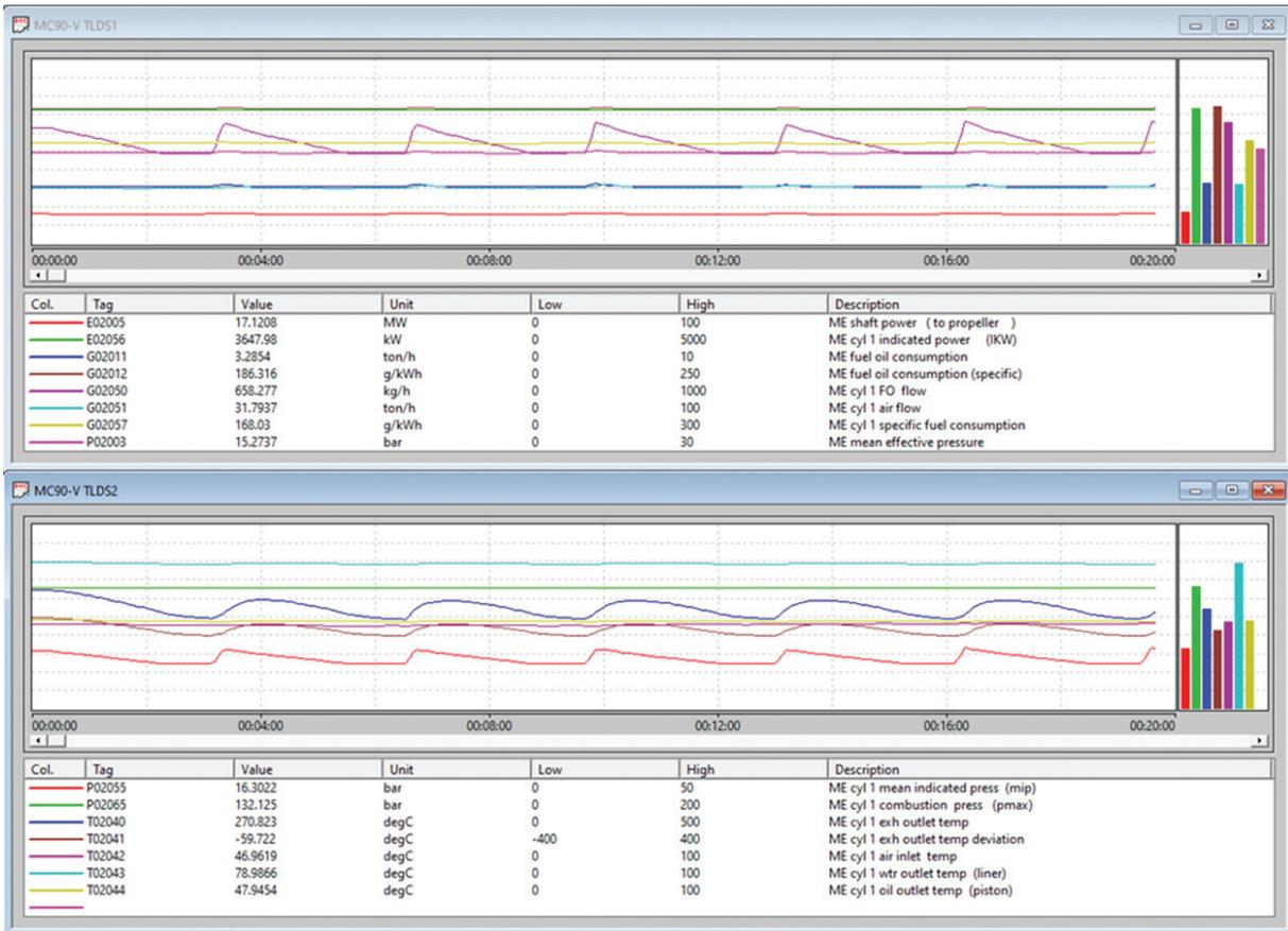
Figure 5 The values of two parameters during a fault condition
