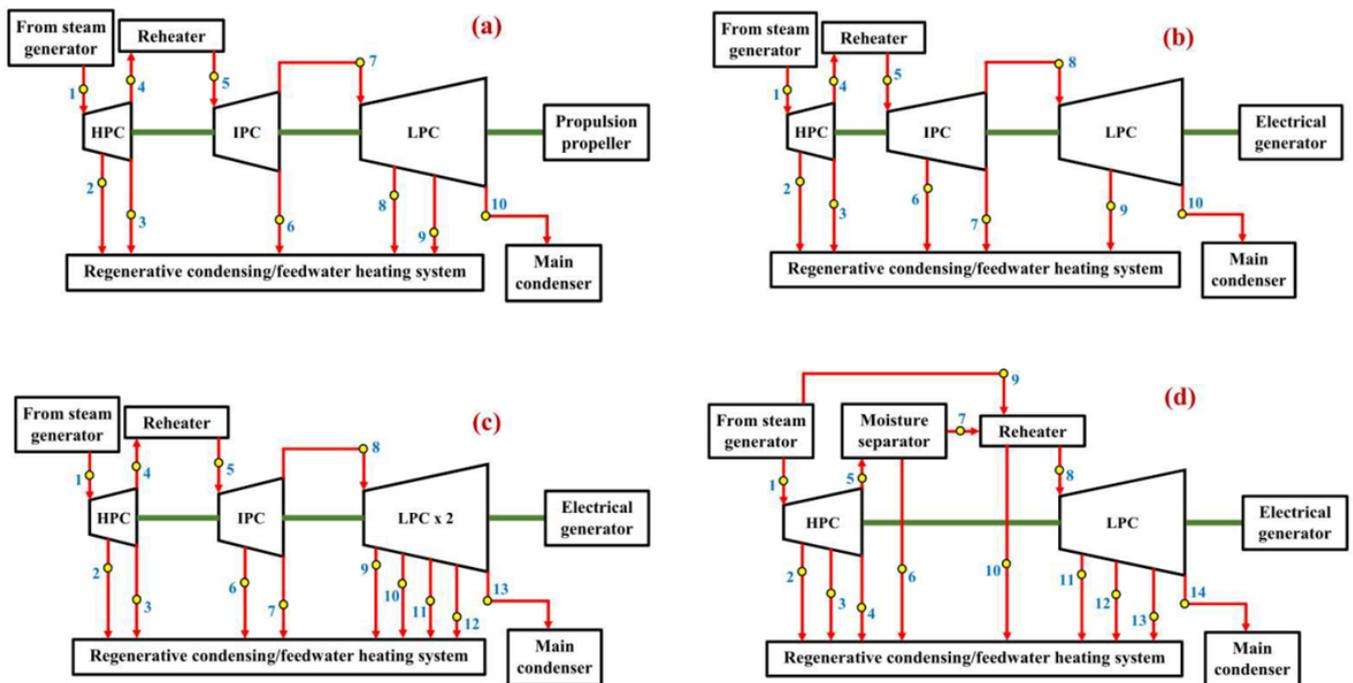
**Fig. 1** General schemes of the observed steam turbines along with operating points required for the analysis:
