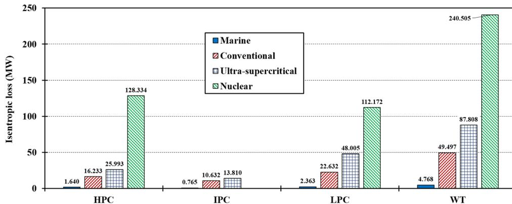
Fig. 5 Isentropic loss of each cylinder and whole turbine
