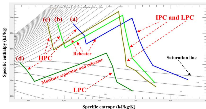
**Fig. 2** Steam expansion and reheating process in  $h$ - $s$  diagram through all cylinders of all analyzed steam turbines: (a) Marine propulsion steam turbine; (b) Steam turbine from the conventional power plant; (c) Steam turbine from ultra-supercritical power plant; (d) Steam turbine from nuclear power plant
