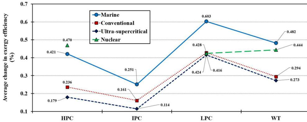
**Fig. 11** Average change in exergy efficiency (between ambient temperatures 5 °C and 45 °C) of each cylinder and whole turbine
