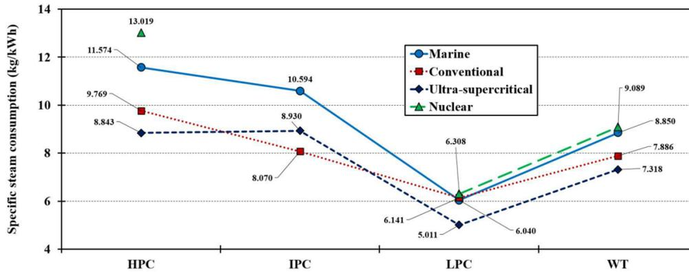
Fig. 9 Specific steam consumption of each cylinder and whole turbine
