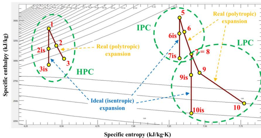
Fig. 3 Comparison of ideal (isentropic) and real (polytropic) steam expansion processes through all cylinders of steam turbine from the conventional power plant
