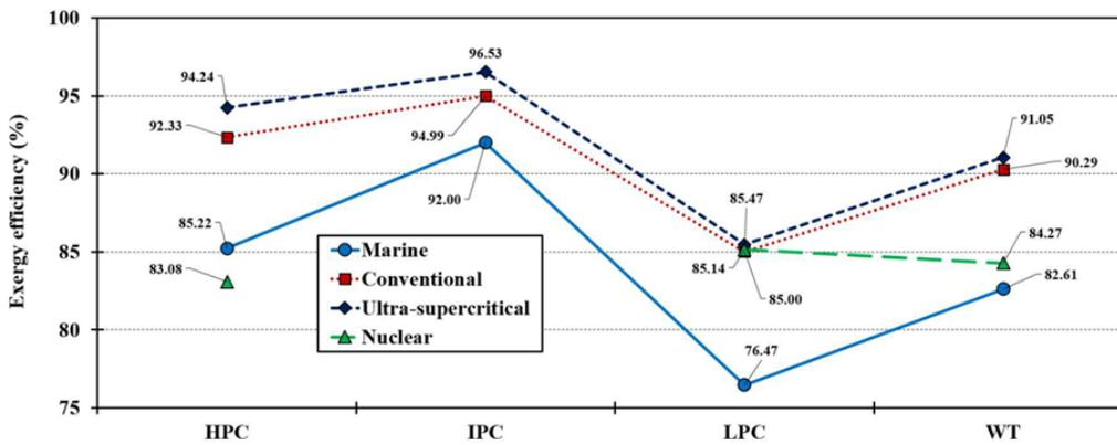
Fig. 8 Exergy efficiency of each cylinder and whole turbine
