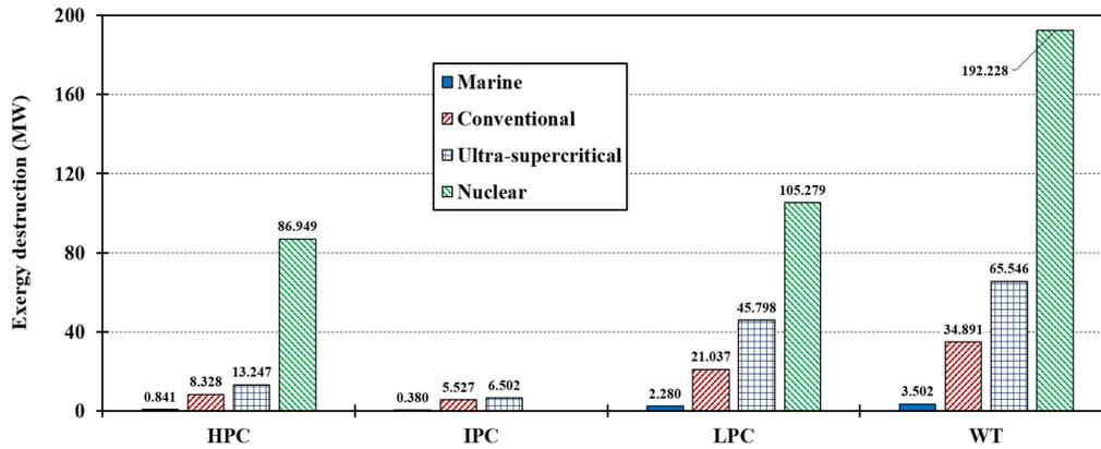
Fig. 7 Exergy destruction of each cylinder and whole turbine
