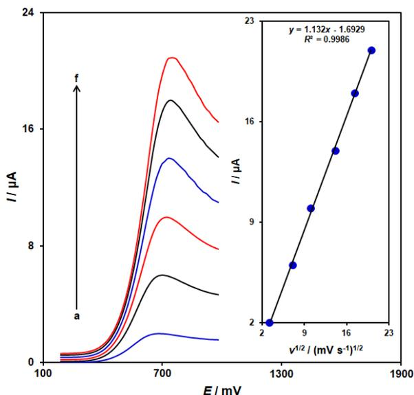
**Figure 2.** Linear sweep voltammograms of vitamin B<sub>6</sub> (100.0 μM) at ZnFe<sub>2</sub>O<sub>4</sub>/SPGE at different scan rates of a) 10, b) 50, c) 100, d) 200, e) 300, and f) 400 mV/s in 0.1 M PBS (pH 7.0). Inset: Plot of *I<sub>p</sub>* versus *v*<sup>1/2</sup> for the oxidation of vitamin B<sub>6</sub> at ZnFe<sub>2</sub>O<sub>4</sub>/SPGE.
