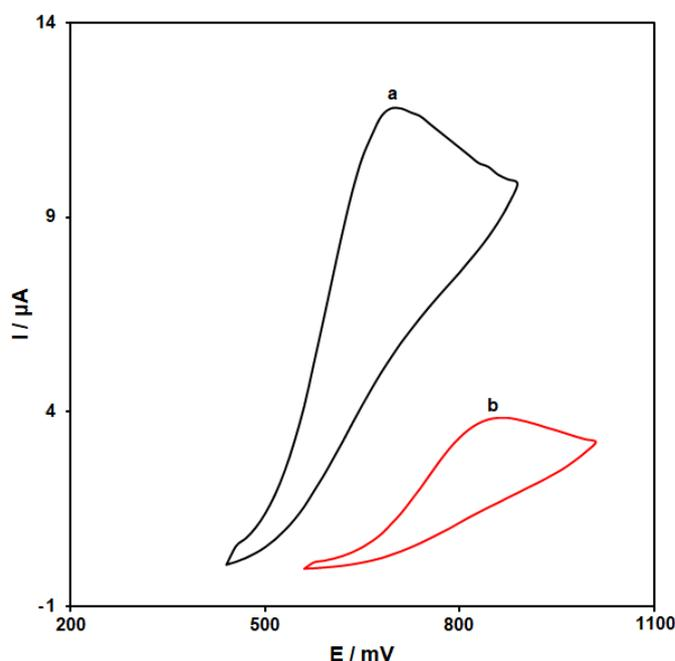
**Figure 1.** Cyclic voltammograms of a) ZnFe<sub>2</sub>O<sub>4</sub>/SPGE and b) SPGE in the presence of 200.0 μM vitamin B<sub>6</sub> at a pH 7.0 of 0.1 M PBS, respectively.
