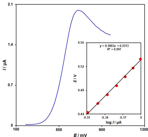
**Figure 3.** Linear sweep voltammogram for ZnFe<sub>2</sub>O<sub>4</sub>/SPGE in the presence of 0.1 M PBS (Ph 7.0) with 100.0 μM of vitamin B<sub>6</sub> at the scan rate of 10 mV/s; Points: outputs used in Tafel plot; Inset: Tafel plot of LSV.
