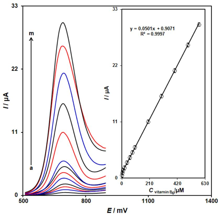
**Figure 5.** DPV curves of ZnFe<sub>2</sub>O<sub>4</sub>/SPGE in the 0.1 M buffer solution (pH 7.0) containing different concentrations of vitamin B<sub>6</sub>. a-m corresponds to 0.8, 5.0, 10.0, 20.0, 40.0, 60.0, 80.0, 100.0, 200.0, 300.0, 400.0, 500.0, and 585.0 μM vitamin B<sub>6</sub>. Inset: Plots of electrocatalytic peak current as a function of vitamin B<sub>6</sub> concentration.
