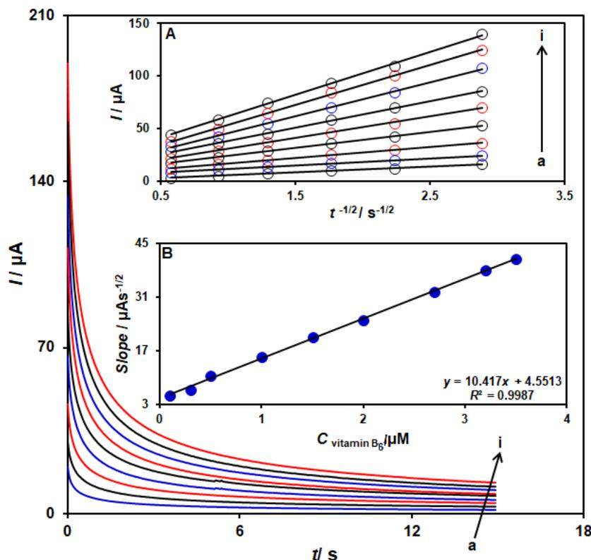
**Figure 4.** Chronoamperograms obtained at the ZnFe<sub>2</sub>O<sub>4</sub>/SPGE in the presence of a) 0.1, b) 0.3, c) 0.5, d) 1.0, e) 1.5, f) 2.0, g) 2.7, h) 3.2, and i) 3.5 μM vitamin B<sub>6</sub> in the 0.1 M buffer solution (pH 7.0). A) Plot of *I* versus *t*<sup>-1/2</sup> for electrooxidation of vitamin B<sub>6</sub> obtained from chronoamperograms a–i. B) Plot of slope from straight lines versus vitamin B<sub>6</sub> level.
