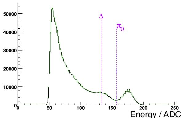
Fig. 5. Energy spectrum measured by the A4 lead fluoride calorimeter. The incident beam energy was 1.5 GeV and a hydrogen target was used. The  $x$  axis shows ADC channels. One can see the peak of elastically scattered electrons around ADC channel 175 which corresponds to an energy of about 1.1 GeV. The pion production threshold and the position of the  $\Delta$  resonance are also indicated..
