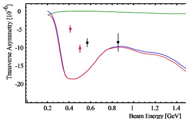
Fig. 7. Transverse asymmetry  $A_{\perp}$  as a function of the beam energy for the A4 experiment at forward angles. The curves show the calculation from [3]: Nucleon ground state only (green), excited intermediate states (blue) and the sum of the two (red). The data points show measurements at MAMI. The points in black are taken from [5], the red points are preliminary.
