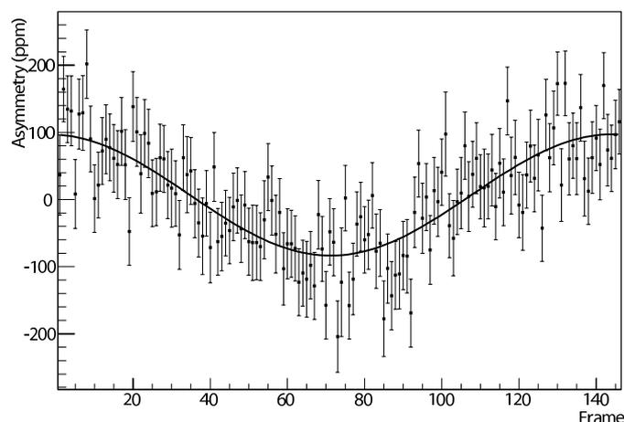
Fig. 6. Measured asymmetries  $A_{\perp}$  at backward angles, hydrogen target and beam energy  $E = 315$  MeV, as a function of the frame number of the calorimeter. The frames cover the whole azimuthal angle, i.e. frame 146 corresponds to  $\phi_e = 2\pi$ .
