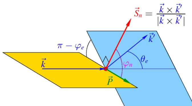
Fig. 3. Scattering of transversely polarized electrons. The incoming momentum is denoted by  $\vec{k}$ , the outgoing by  $\vec{k}'$ . The scattering plane is shown in blue, the vector  $\vec{S}_n$  is normal vector of the scattering plane. The spin of the electron before the scattering is shown by  $\vec{P}$ .
