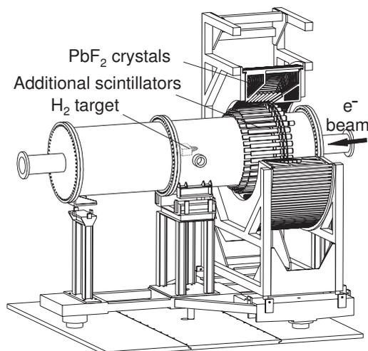
Fig. 4. Drawing of the A4 lead fluoride calorimeter and the scattering chamber [12]. The calorimeter is mounted on a rotatable platform so that one can easily change between forward and backward angle configuration. The backward angle configuration is shown here. The lead fluoride crystals cover the  $2\pi$  azimuthal range. Between the crystals and the scattering chambers are plastic scintillators installed which allow a separation of neutral and charged particles.
