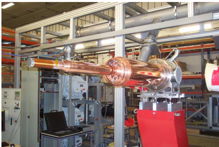
Fig. 4. The new dilution refrigerator for the Crystal Ball Frozen Spin Target.
