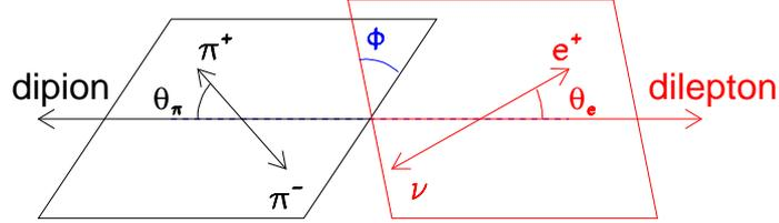
Fig. 1. Topology of the  $K^\pm \rightarrow \pi^+ \pi^- e^\pm \nu$  decay showing the angle definitions.
