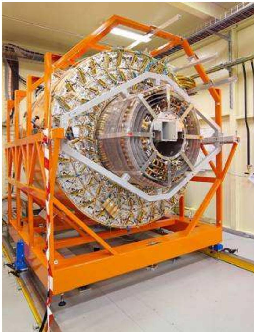
*Fig. 2. The pre-assembled TRT-SCT package for the barrel part of the Inner Detector.*
