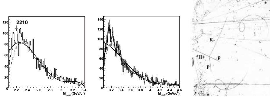
Fig. 3. a)  $\Lambda p$  spectrum for relativistic positive tracks in the range of  $P_p > 1.5 \text{ GeV}/c$  with bin size of  $15 \text{ MeV}/c^2$ ; b)  $\Lambda pp$  spectrum for identified protons with bin size of  $16 \text{ MeV}/c^2$ ; c) The weak decay for  $H^+ \rightarrow K^- pp$ . The dashed histogram shows simulated events by FRITIOF. The experimental background is shown by the solid curve.
