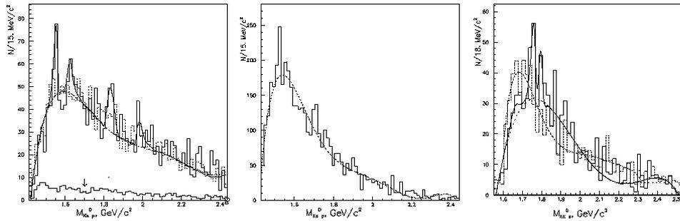
Fig. 4. a)  $K_s^0 p$  spectrum for identified protons in the range of  $0.35 < P_p < 0.90$  GeV/c ( $\overline{K_s^0 p}$  comb. by FRITIOF - lower histogram); b) ( $K_s^0$ , pos. relativistic tracks) spectrum in the momentum range of  $0.9 < P_p < 1.7$  GeV/c; c)  $K_s^0 \Lambda$  spectrum. The dashed histogram shows simulated events by FRITIOF.
