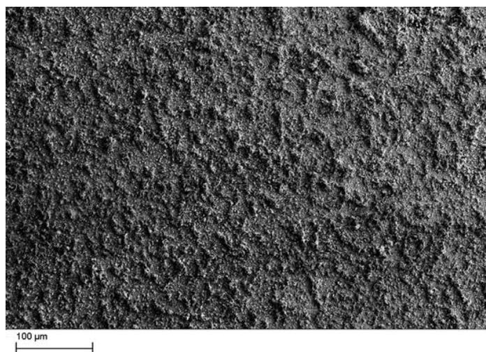
**Figure 5.** SEM image of Re-Mo thin film deposited on Pt electrode (production of rhenium-molybdenum alloys containing 45-80 wt.% Re from 0.0015 M  $\text{Na}_2\text{MoO}_4$  + 0.0035 M  $\text{KReO}_4$  + 2M  $\text{H}_2\text{SO}_4$ ; pH 0.4;  $t = 75^\circ\text{C}$ )
