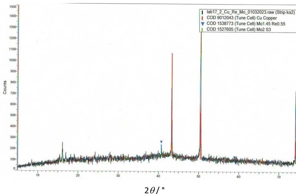
**Figure 7.** X-ray pattern of deposited Re-Mo thin film on Pt electrode and annealed at 500 °C for 2 hours (production of rhenium-molybdenum alloys containing 45-80 wt.% Re from 0.0015 M  $\text{Na}_2\text{MoO}_4$  + 0.0035 M  $\text{KReO}_4$  + 2 M  $\text{H}_2\text{SO}_4$ ; pH 0.4;  $t = 75^\circ\text{C}$ )
