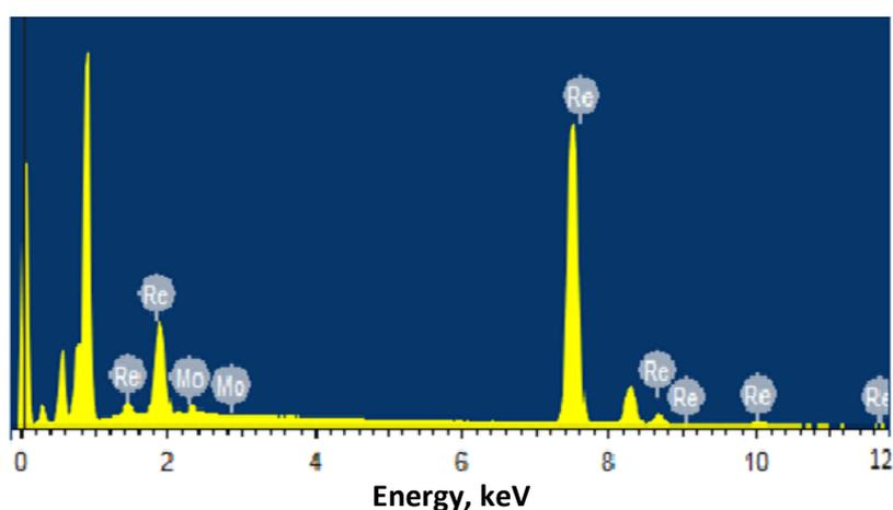
**Figure 6.** Elemental analysis of Re-Mo thin film deposited on Pt electrode (production of rhenium-molybdenum alloys containing 45-80 wt.% Re from 0.0015 M  $\text{Na}_2\text{MoO}_4$  + 0.0035 M  $\text{KReO}_4$  + 2M  $\text{H}_2\text{SO}_4$ ; pH 0.4;  $t = 75^\circ\text{C}$ )
