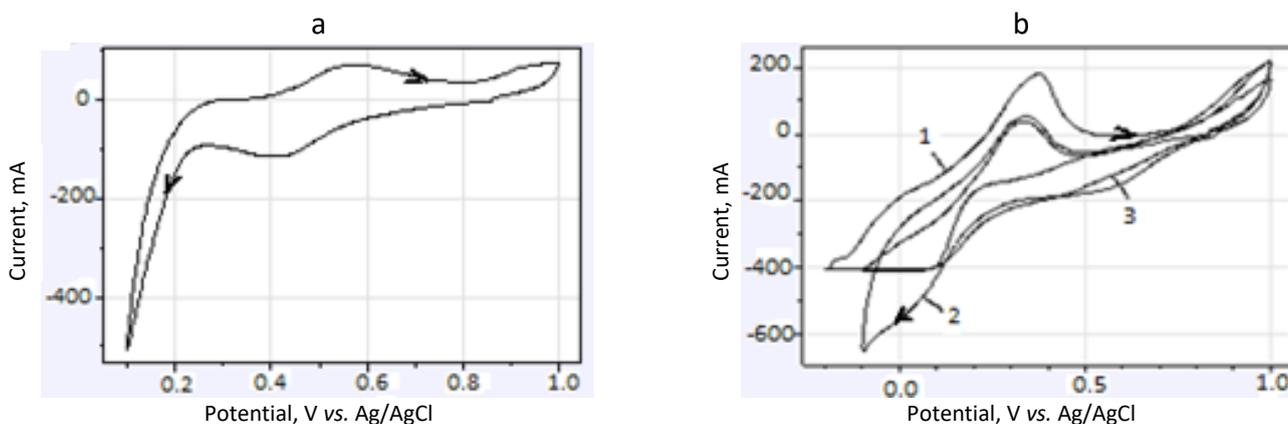
**Figure 3.** Cyclic voltammograms ( $5\text{ mV s}^{-1}$ ) of rhenium and molybdenum co-deposition on Pt electrode in  $2\text{ M H}_2\text{SO}_4$ , pH 0.4,  $75\text{ }^\circ\text{C}$ , in presence of  $0.0015\text{ M Na}_2\text{MoO}_4$  and: (a)  $0.035\text{ M KReO}_4$ ; (b) various concentrations of  $\text{KReO}_4$  (1)  $0.035\text{ M}$ ; (2)  $0.0035\text{ M}$ ; (3)  $0.00069\text{ M}$
