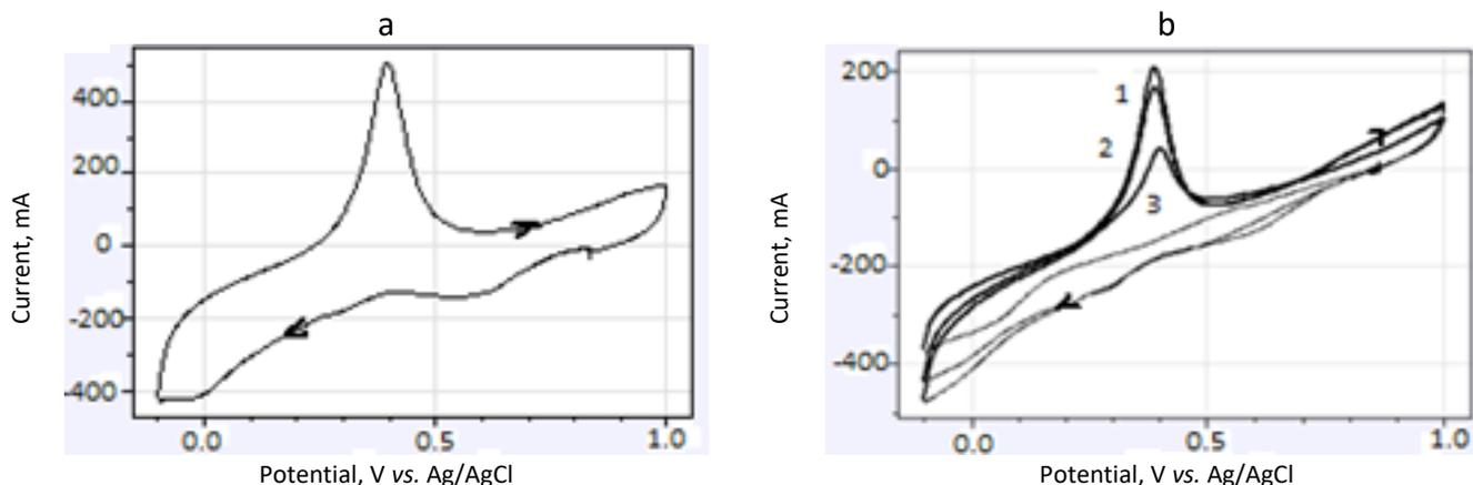
**Figure 2.** Cyclic voltammograms ( $5 \text{ mV s}^{-1}$ ) of rhenium deposition on Pt electrode in  $2 \text{ M H}_2\text{SO}_4$ ,  $\text{pH } 0.4$ ,  $75^\circ\text{C}$  and presence of: (a)  $0.00084 \text{ M KReO}_4$  and (b) various concentrations of  $\text{KReO}_4$  (1)  $0.00069 \text{ M}$ ; (2)  $0.0035 \text{ M}$ ; (3)  $0.035 \text{ M}$
