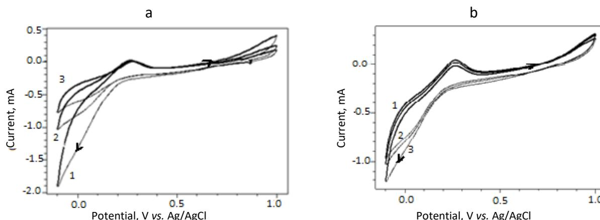
**Figure 1.** Cyclic voltammograms of molybdenum deposition on Pt electrode in 2 M H<sub>2</sub>SO<sub>4</sub>, pH 0.4, 75 °C at: (a) scan rate 5 mV s<sup>-1</sup> and following concentrations of Na<sub>2</sub>MoO<sub>4</sub> (1) 0.02 M; (2) 0.015 M; (3) 0.0015 M and (b) 0.0015 M Na<sub>2</sub>MoO<sub>4</sub> at different cycles (1-3)
