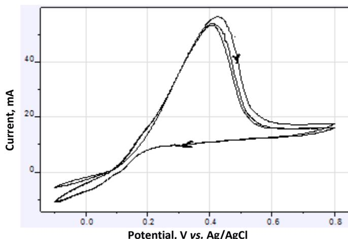
**Figure 4.** Cyclic voltammograms ( $5 \text{ mV s}^{-1}$ ) of Ni working electrode in  $2 \text{ M H}_2\text{SO}_4$ ,  $0.0015 \text{ M Na}_2\text{MoO}_4$  and  $0.0035 \text{ M KReO}_4$ , pH 0.4;  $75 \text{ }^\circ\text{C}$
