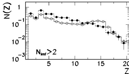
Fig. 6.  $^{32}\text{S} + ^{58}\text{Ni}$  reaction at 11 A MeV. Filtered CMD charge distribution for events with at least three IMFs: open symbols refer to events detected in the whole apparatus, full symbols to events detected in GARFIELD. As shown in Fig. 4, this results in  $\langle b \rangle \approx 2$  fm. Both charge distributions are normalized to the total number of events.
