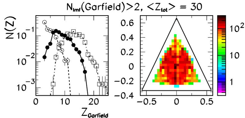
Fig. 7.  $^{32}\text{S} + ^{58}\text{Ni}$  reaction at 11 A MeV. Charge distribution of the three largest IMFs detected in each event (left panel) and relative Dalitz plot for the experimental data. Both charge distributions are normalized to the total number of events.
