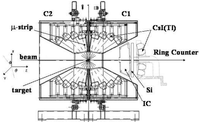
Fig. 1. Schematic drawing of the experimental apparatus: the two drift chambers (C1 and C2) are located back to back, with the target in between, while the annular detector is positioned in the forward direction with respect to the beam.
