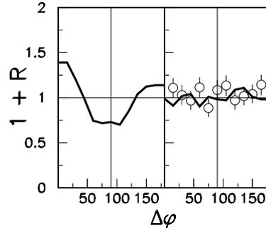
Fig. 3.  $^{32}\text{S} + ^{58}\text{Ni}$  reaction at 11 A MeV. Azimuthal correlation function for  $\alpha$ -particles detected in GARFIELD, gated by three IMFs detected at large angles in the GARFIELD drift chamber. Left panel: correlation function calculated with the sequential statistical model code GEMINI for  $\langle L \rangle = 48 \text{ h}$ . Right panel: experimental data and GEMINI calculation for  $\langle L \rangle = 10 \text{ h}$ .
