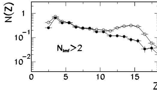
Fig. 5.  $^{32}\text{S} + ^{58}\text{Ni}$  reaction at 11 A MeV. Charge distribution of IMFs detected in the whole apparatus (open symbols) and in GARFIELD (full symbols) for events with at least three IMFs. Both charge distributions are normalized to the total number of events.
