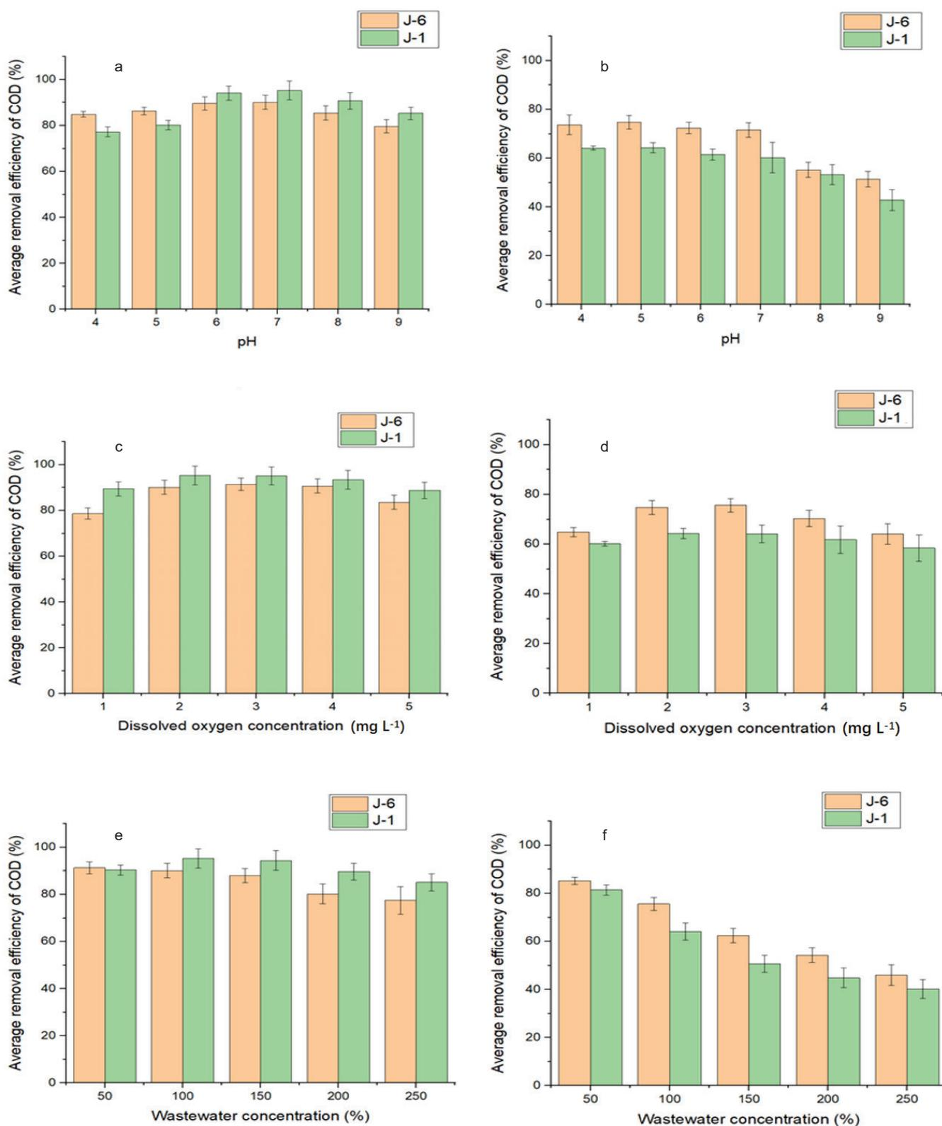
Fig. 3 – Effect of different factors on the treatment of lignin-containing wastewater (a: effect of pH on traditional Chinese medicine wastewater treatment; b: effect of pH on papermaking wastewater treatment; c: effect of DO on traditional Chinese medicine wastewater treatment; d: effect of DO on papermaking wastewater treatment; e: effect of wastewater concentration on traditional Chinese medicine wastewater treatment; f: effect of wastewater concentration on papermaking wastewater treatment)
