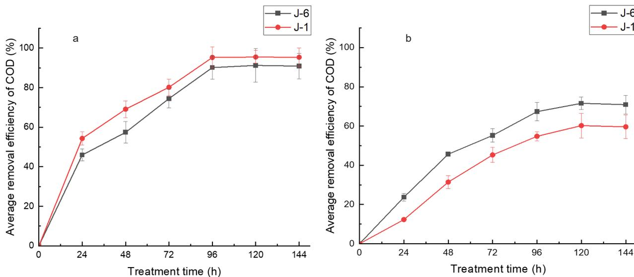
Fig. 1 – Effect of treatment time on lignin-containing wastewater treatment (a: traditional Chinese medicine wastewater; b: paper-making wastewater)
