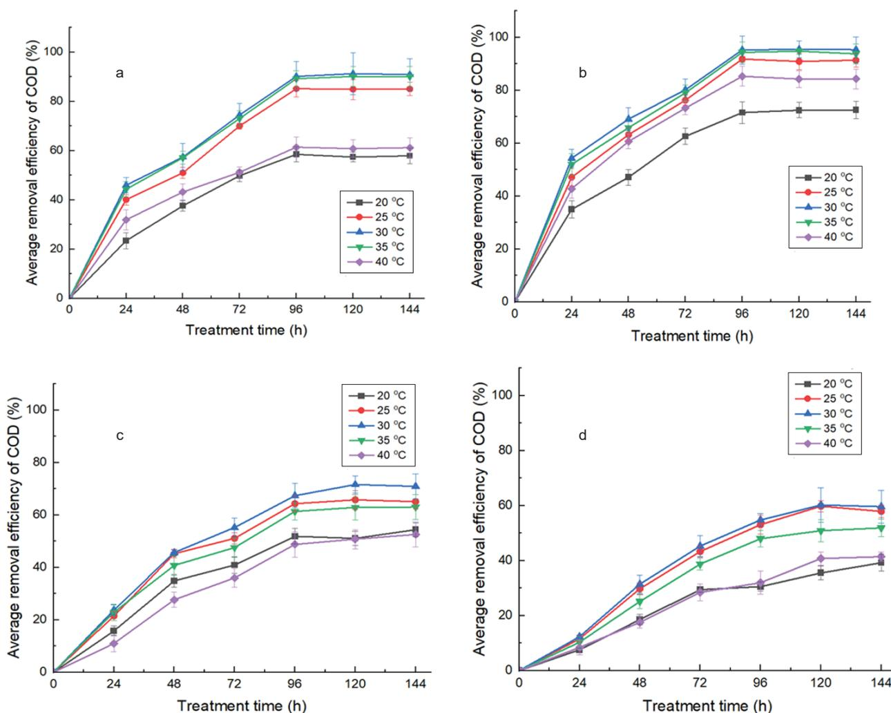
Fig. 2 – Effect of temperature on lignin-containing wastewater treatment (a: traditional Chinese medicine wastewater treatment by J-6; b: traditional Chinese medicine wastewater treatment by J-1; c: papermaking wastewater treatment by J-6; d: papermaking wastewater treatment by J-1)
