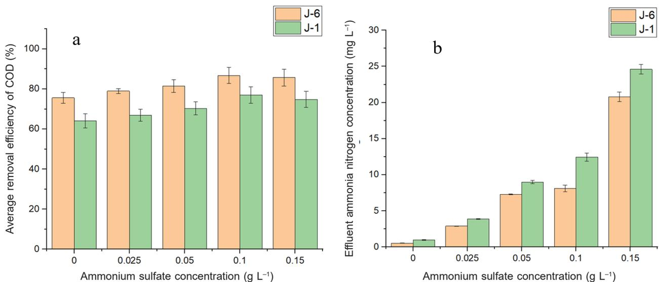
Fig. 4 – Effect of nitrogen source addition on papermaking wastewater treatment (a: average removal efficiency of COD under different nitrogen addition; b: effluent ammonia nitrogen concentration under different nitrogen addition)
