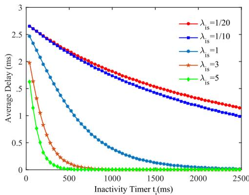
Fig. 11. Average Delay under different Inactivity Timers.
