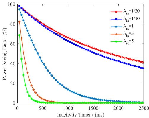
Fig. 7. Power Saving Factor versus inactivity time with different  $\lambda_{is}$ .
