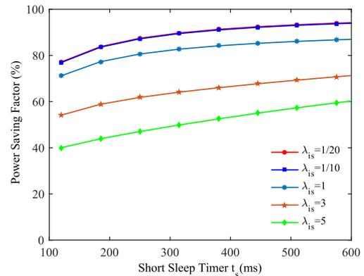
Fig. 8. Power Saving Factor versus Short Sleep Timers.
