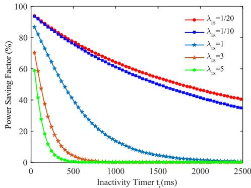
Fig. 6. Power Saving Factor versus inactivity time with different  $\lambda_{is}$ .
