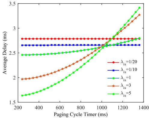
Fig. 10. Average Delay under different Paging Cycle Timers.
