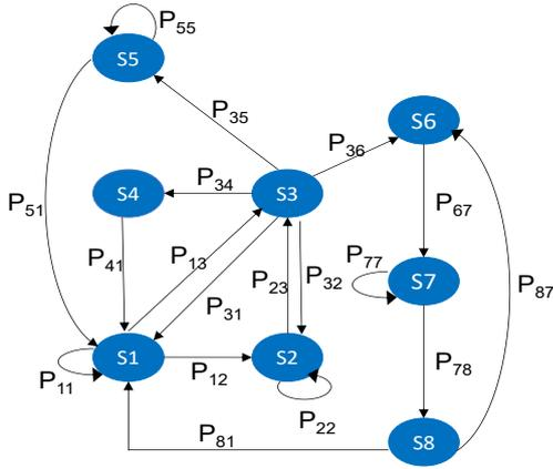
Fig. 4. Semi-Markov chain diagram for the proposed DRX-BM.
