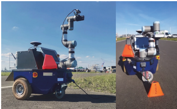
Figure 3 Coning robot and cone placing
