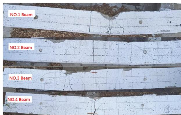
Figure 8 Diagram of experimental beam failure
