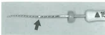
Slika 21. Sjajna mrlja (eng. the shiny spot) (preuzeto iz Deutsch AS. Broken Endodontic Instruments: Watch out!. (monograph on the Internet). New York: Musikant, Deutsch, Kase, Dukoff, Bui, Lipner & Kim., 2000 (2008 Dec 4). Available from: http://www.Endomail.com/articles/asdo1brokeninst.html )
