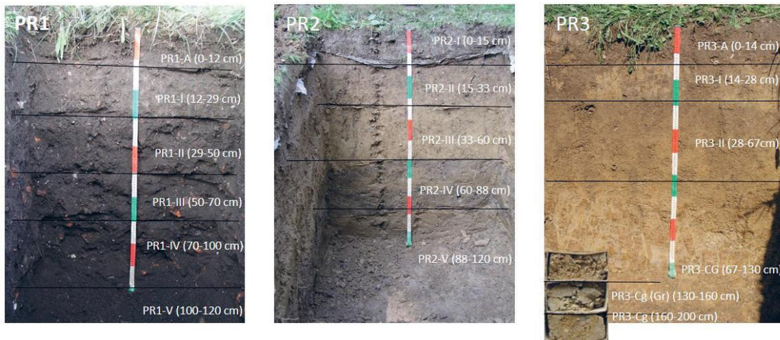
Figure 4. Urban soil profiles PR1, PR2 and PR3 with their determined horizons/layers.
