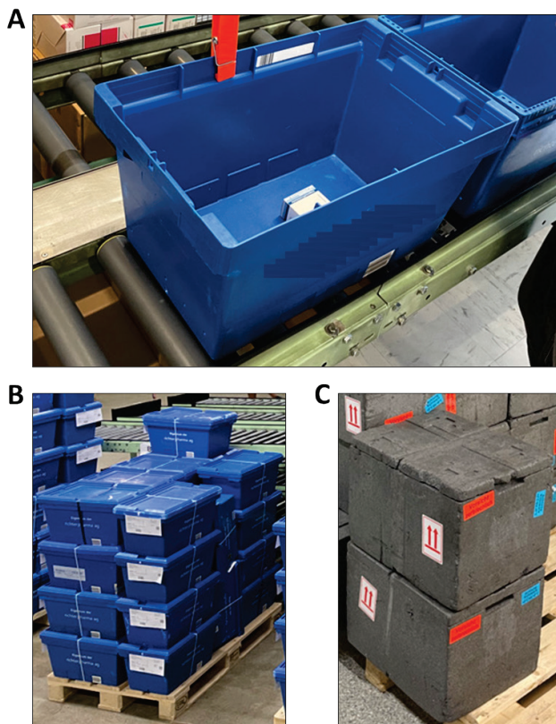
Figure 7 Transport items currently in use by the wholesaler. (A) An RTI with the lid removed. These types of RTIs are used for transportation of drugs that need no cooling. (B) Stacked RTIs. (C) Polystyrene-based cooling boxes to be filled with dry ice for cold chain delivery. RTI, returnable transport item.
