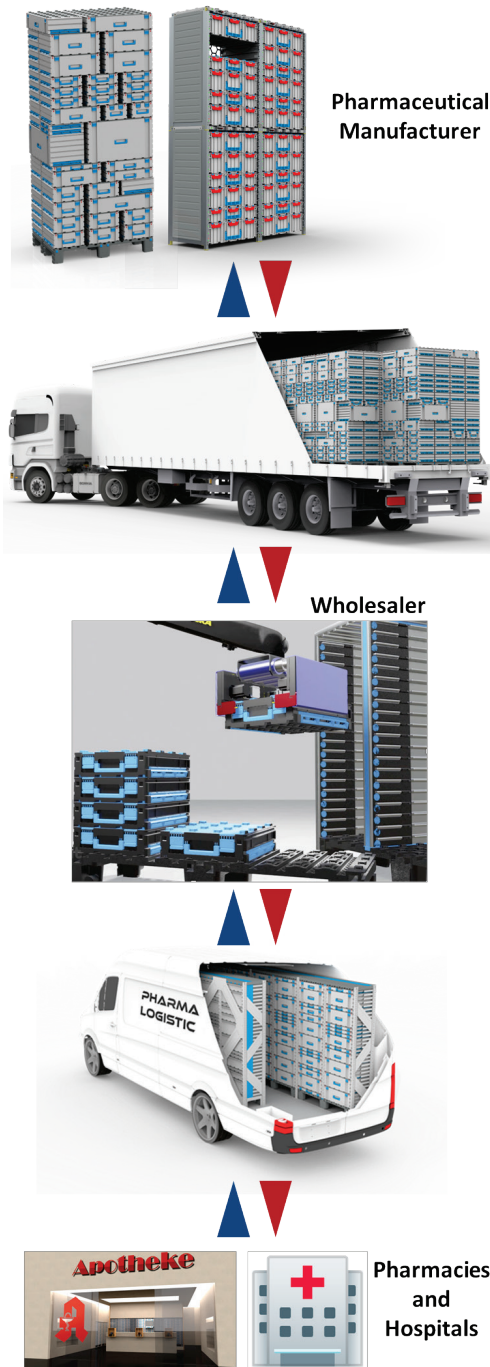
Figure 2 The vision of DigiPharmaLogNet. The RTI solution to be developed by the project team has a modularity mechanism incorporated, which allows stacking boxes with different sizes. Its compatibility with a robotic system enables automation of warehouse processes. Since RTIs are intended for reuse, circular logistic chains could be established in pharma logistics. RTI, returnable transport item.
