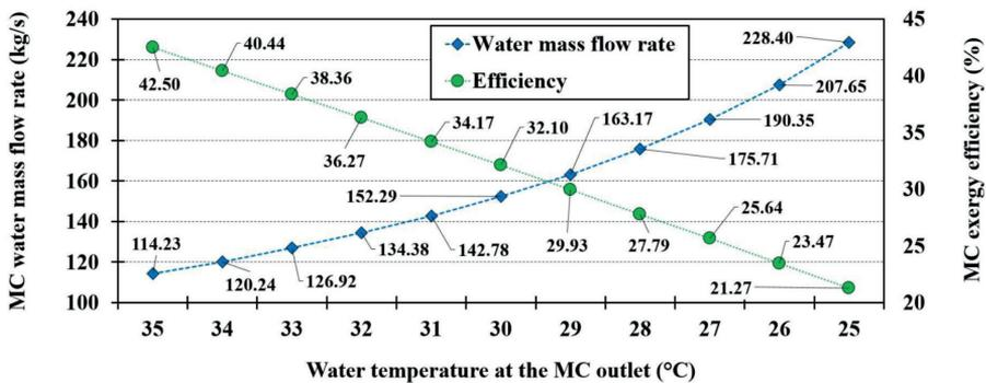
Figure 7 - The change in MC water mass flow rate and exergy efficiency during the change in water temperature at the MC outlet
