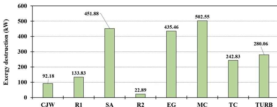
Figure 5 - Exergy destruction of all components from the observed waste heat recovery supercritical CO<sub>2</sub> system (CJW - Cooling Jacket Water waste heat exchanger; R1- Recuperator 1; SA - Scavenge Air waste heat exchanger; R2 - Recuperator 2; EG – Exhaust Gas waste heat exchanger; MC – Main Cooler; TC – Turbocompressor; TURB – Turbine)
