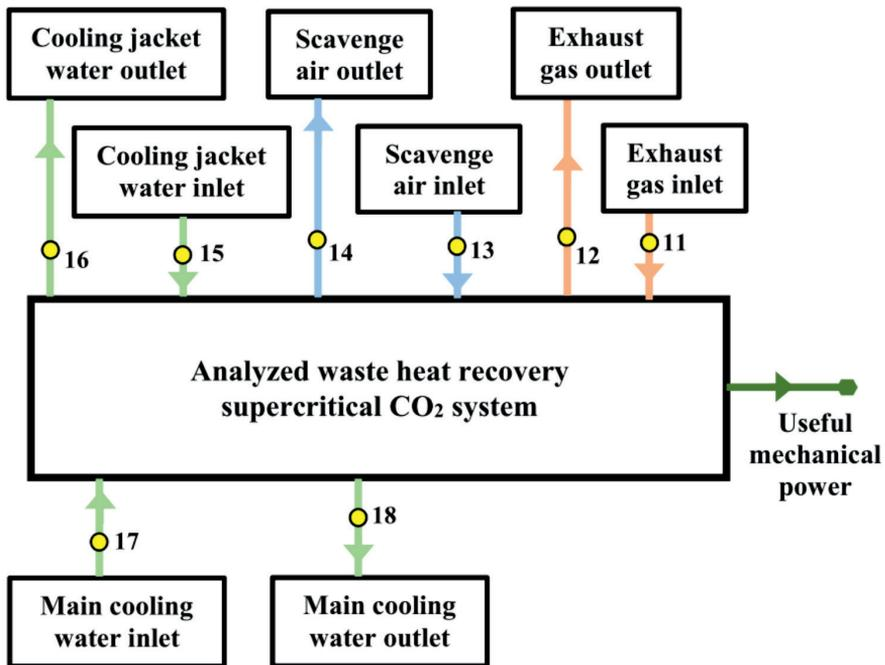
Figure 2 - Scheme for exergy analysis parameters definition of the whole observed waste heat recovery supercritical CO<sub>2</sub> system
