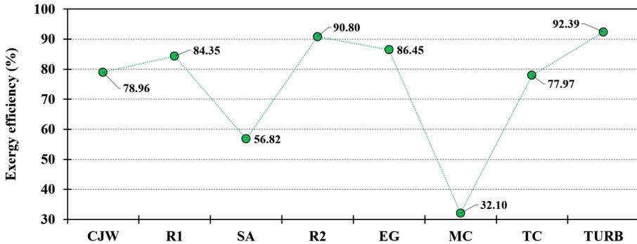
Figure 6 - Exergy efficiency of all components from the observed waste heat recovery supercritical CO<sub>2</sub> system (CJW - Cooling Jacket Water waste heat exchanger; R1- Recuperator 1; SA - Scavenge Air waste heat exchanger; R2 - Recuperator 2; EG – Exhaust Gas waste heat exchanger; MC – Main Cooler; TC – Turbocompressor; TURB – Turbine)
