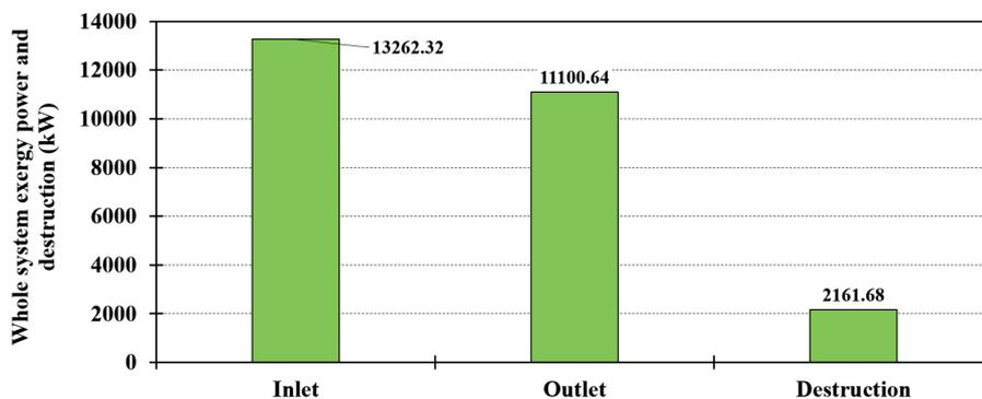
Figure 9 – Exergy power inlet, outlet and destruction of the whole observed waste heat recovery supercritical CO<sub>2</sub> system
