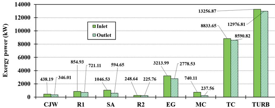
Figure 4 - Exergy power inlet and outlet of all components from the observed waste heat recovery supercritical CO<sub>2</sub> system (CJW - Cooling Jacket Water waste heat exchanger; R1- Recuperator 1; SA - Scavenge Air waste heat exchanger; R2 - Recuperator 2; EG – Exhaust Gas waste heat exchanger; MC – Main Cooler; TC – Turbocompressor; TURB – Turbine)
