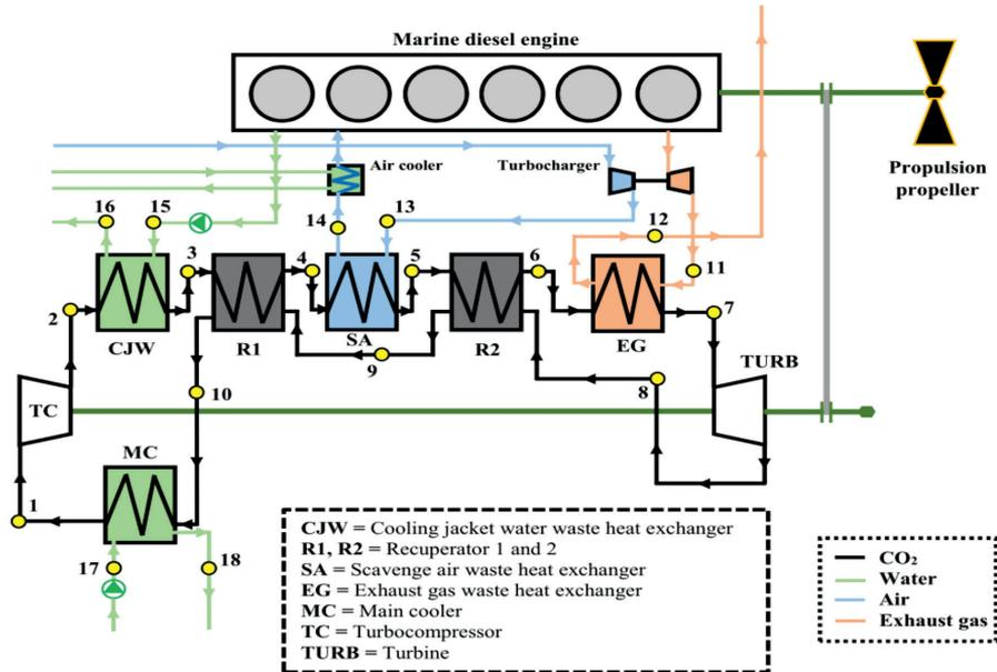
Figure 1 – General scheme of the observed waste heat recovery supercritical CO<sub>2</sub> system with marked operating points required for the exergy analysis
