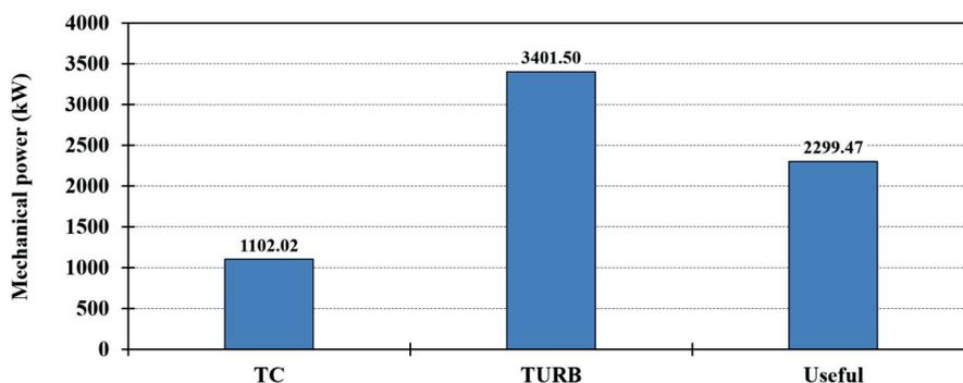
Figure 3 - Produced (turbine), used (turbocompressor) and useful mechanical power from the observed waste heat recovery supercritical CO<sub>2</sub> system
