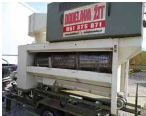
Slika 4. Cilindrični bubanj s tri mreže za čišćenje sjemena blago je nagnut prema dolje (gledano u smjeru čišćenja). Figure 4 Cylindrical drum with three nets for seed cleaning is slightly inclined downwards (viewed in the direction of cleaning).
