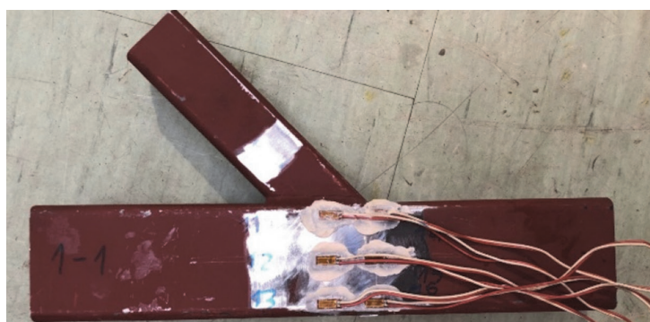
Figure 14. Arrangement of strain gauges on the specimen without damage (Y-joint_ND)
