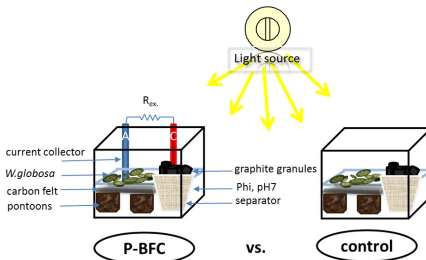
**Figure 1.** Scheme of the experimental setup. The duckweed was grown under polarization conditions of the biofuel cell and compared with plants grown as a control without connection in an electrical circuit
