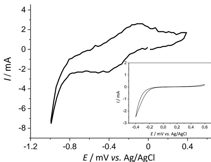
**Figure 4.** Cyclic voltammogram of the *W. globosa* - P-BFC –anolyte (phosphate buffer, pH 7.0) on the 12<sup>th</sup> day of operation. Inset - negative control toward polarization. Scan rate: 10 mV s<sup>-1</sup>, the second scan
