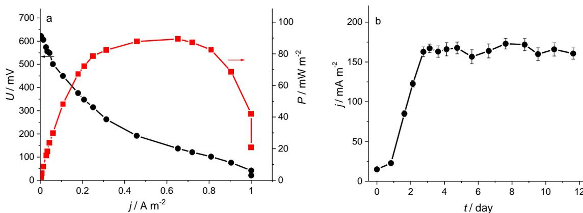
**Figure 3.** (a) Polarization ( $U$  as a function of  $j$ ) and power ( $P$  as a function of  $j$ ) curves of *W. globosa* - P-BFC on the 6<sup>th</sup> day of operation, (b) current density recorded during P-BFC operation across an external load of  $1 \text{ k}\Omega$
