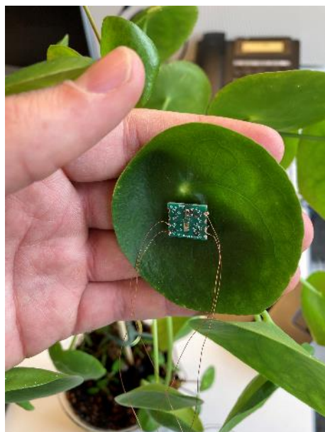
Figure 6. Leaf wetness sensor on a pilea peperomioides leaf
