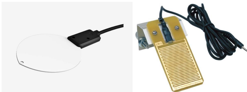
Figure 4. State of the leaf wetness sensor. Left: capacitive sensor (Metergroup) [17]; Right: resistive sensor (Spectrum) [18]
