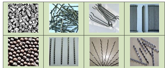
Figure 1: Schematic of steel fibers in different shapes
