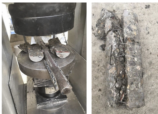
a. Failure mode of plain concrete b. Failure mode of steel fiber concrete
