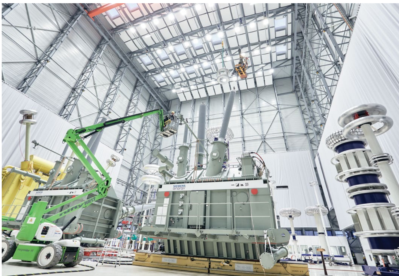
Figure 2. For the German high-voltage direct-current project ULTRANET, Siemens Energy is supplying transformers with carbon-reduced steel from thyssenkrupp Electrical Steel
