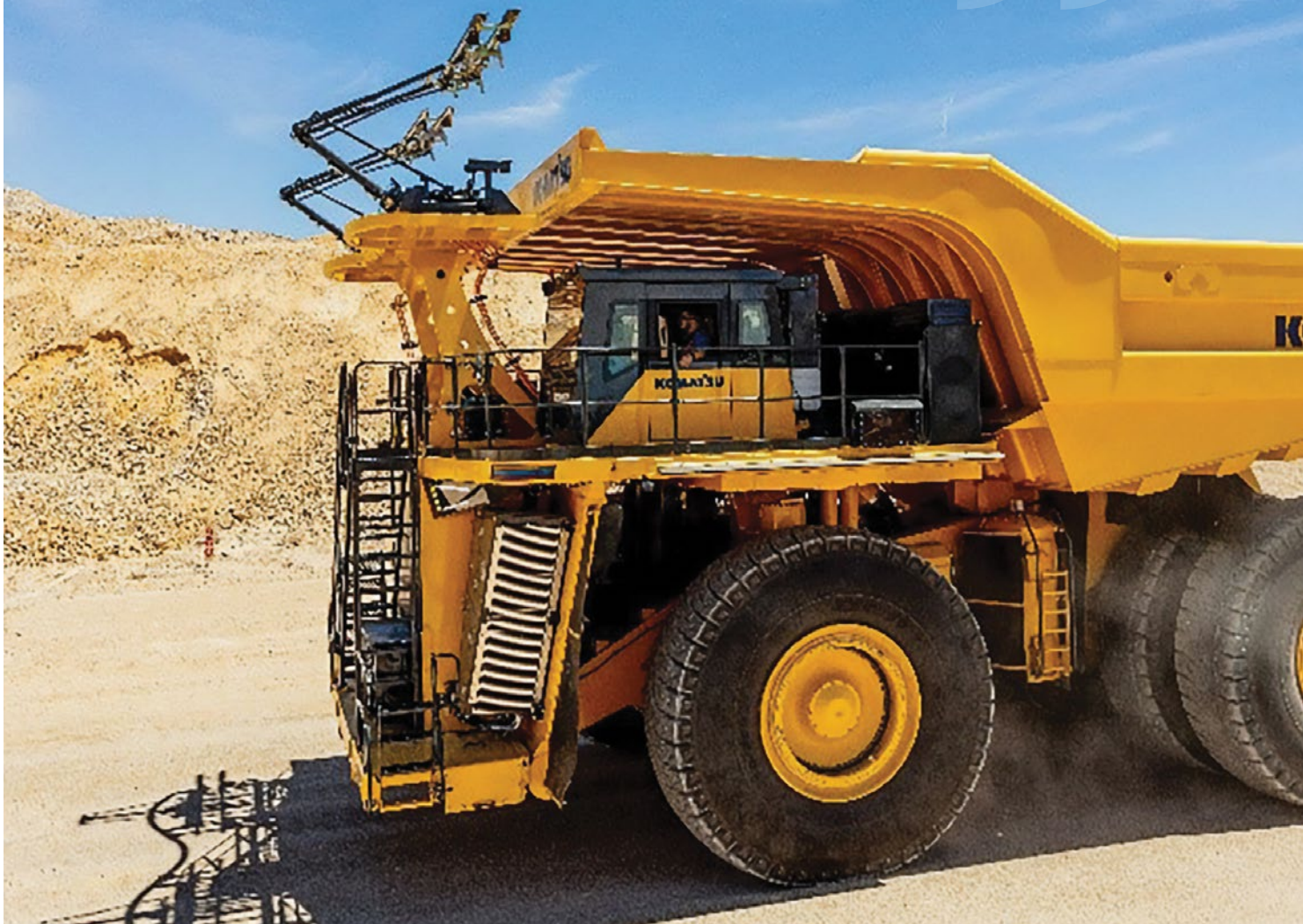
Fig. 4. Power-agnostic truck from Komatsu
